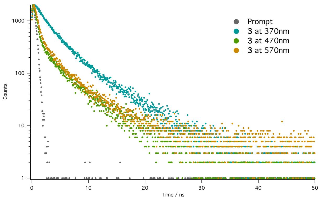
**Figure S4:** Emission lifetimes of compound **3** in RT ACN at room temperature at different wavelengths: all reported decays are multiexponential.
