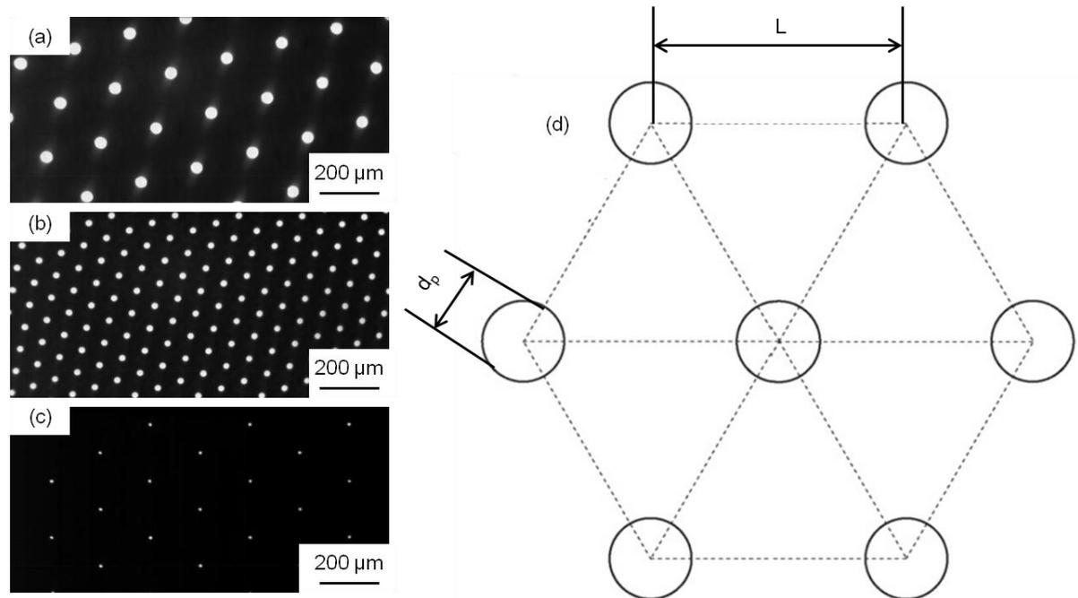
**Figure S1.** Microscopic images of some membranes used in this study: (a)  $d_p = 40 \mu\text{m}$ ,  $L = 200 \mu\text{m}$ , (b)  $d_p = 20 \mu\text{m}$ ,  $L = 80 \mu\text{m}$ , and (c)  $d_p = 10 \mu\text{m}$ ,  $L = 200 \mu\text{m}$ . (d) Schematic view of the pore arrangement showing a regular hexagonal array of cylindrical pores with uniform pore spacing ( $L$  – pore spacing,  $d_p$  – pore diameter).
