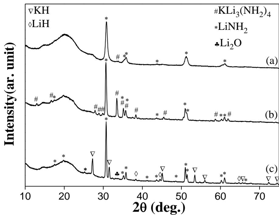
Fig. S1: XRD patterns of the 5 mol% KH-doped  $\text{LiNH}_2$  after ball milling (a) and treatment under Ar (b) and  $\text{H}_2$  (c) flow condition at 200 °C for 4 hours.
