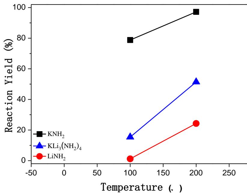
Fig. S2: Reaction yield of the reaction between MNH<sub>2</sub> (M = Li or K) and H<sub>2</sub> at different temperatures for 4 hours.
