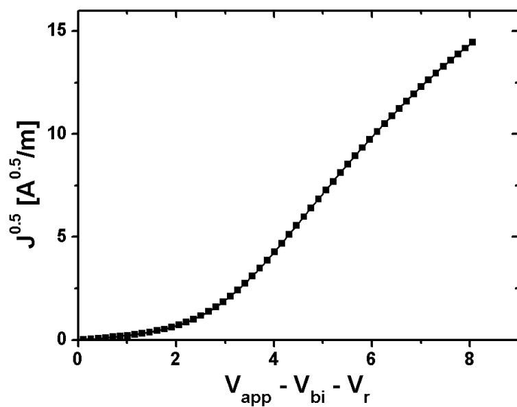
**Fig. S7**  $J^{0.5}$  vs V plot of the hole-only devices based on PBDT-CT:PC<sub>61</sub>BM.
