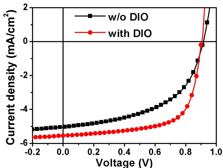
**Fig. S10** *J-V* curves of polymer solar cell based on PBDT-CT:PC<sub>61</sub>BM without and with DIO.
