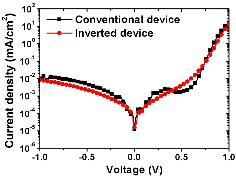
**Fig. S9** Dark current density of polymer solar cell based on PBDT-CT:PC<sub>61</sub>BM.
