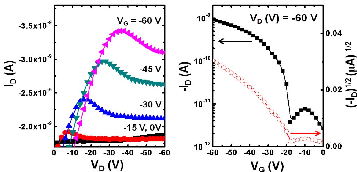
**Fig. S6** Field effect transistor (FET) properties of PBDT-CT.
