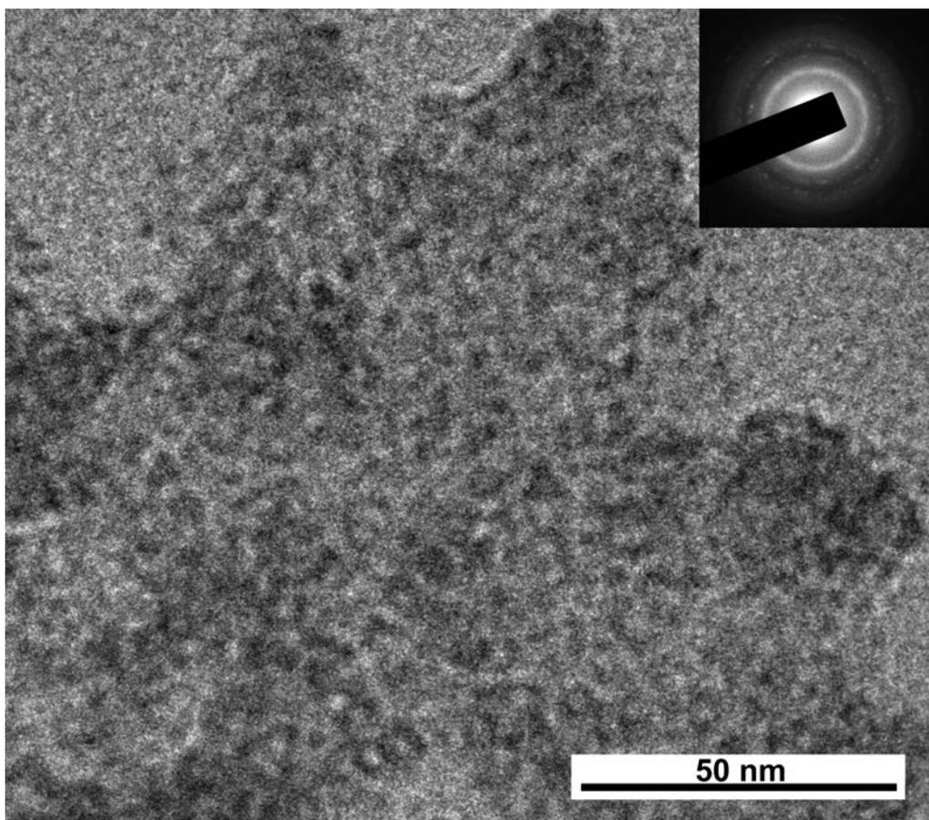
**Figure S3.** TEM image and selected area electron diffraction (SAED) pattern of CP[5]A@QD oligomer.
