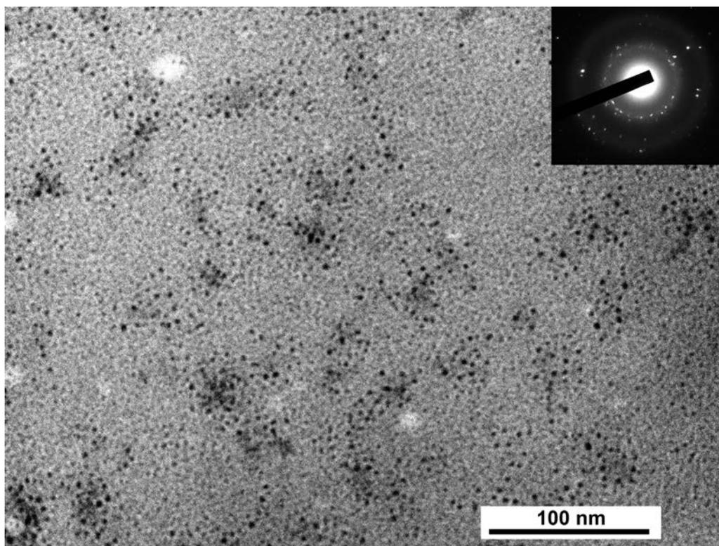
**Figure S1.** TEM image and selected area electron diffraction (SAED) pattern of CP[5]A@QDs.
