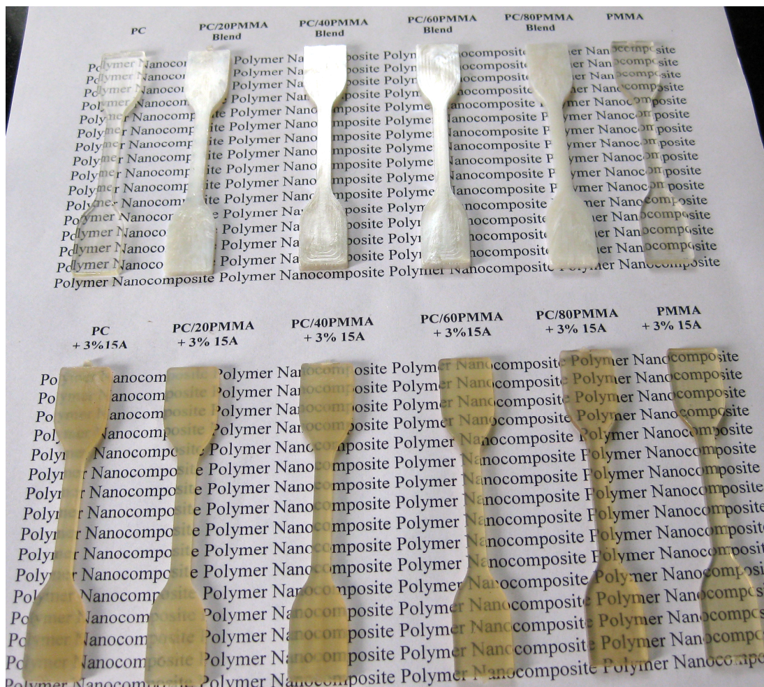
Figure S4: Digital photograph of tensile test specimens of pristine and C15A nanoclay modified PC/PMMA blends, showing optical transparency.
