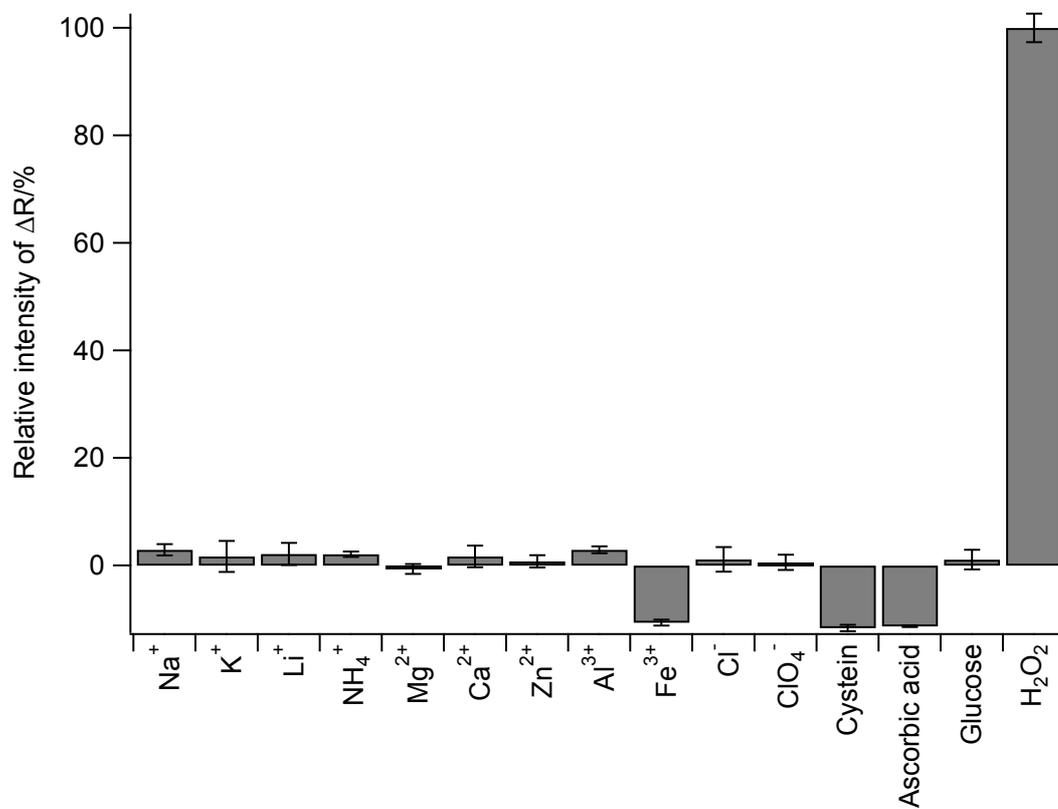
**Figure S-3.** Normalized colourimetric signal induced by the application of 1.0 mM solutions of various foreign species and  $\text{H}_2\text{O}_2$  (error bars:  $n=5$ ). All cations have been applied as nitrate salts.
