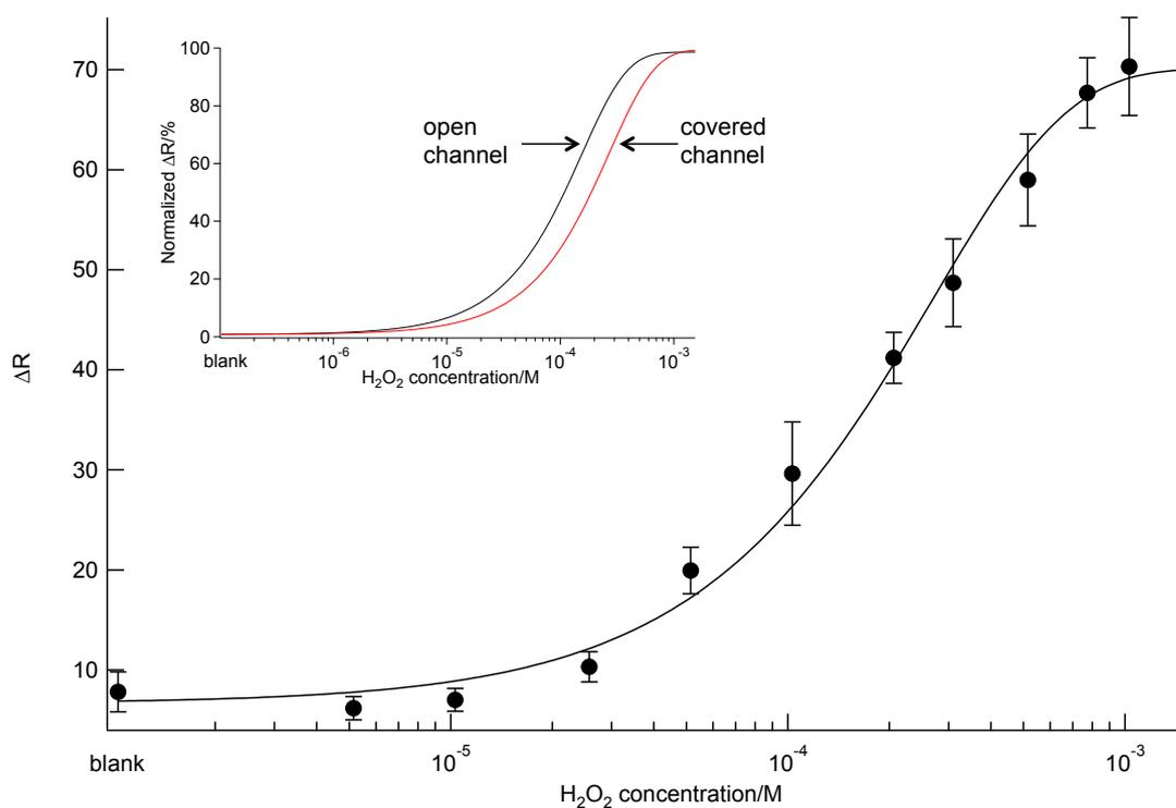
**Figure S-5.** “All-inkjet printed”  $H_2O_2$  sensor with covered tunnel-like channels: the calibration curve was obtained by digital colour analysis using the RGB colour space (error bars:  $n=5$ ).  $\Delta R$  indicates the difference of the R-value between the sample inlet area and the signal detection area; the inset shows the shift of the calibration curve to higher concentrations in the case of using  $\mu$ PADs with covered channels (red line) compared to open channels (black line).
