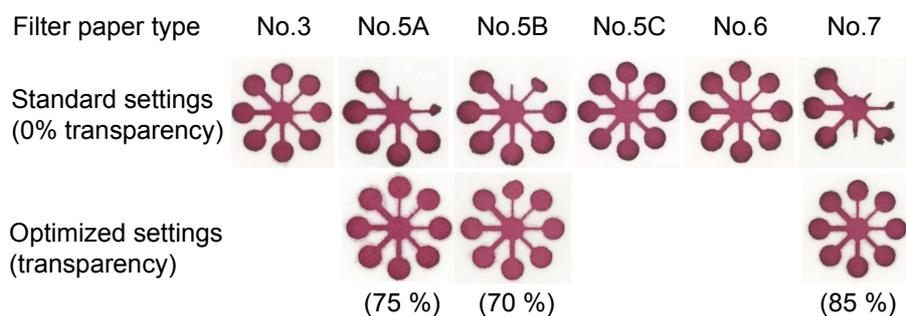
**Figure S-2.** Microfluidic structures printed on various types of filter papers. For details regarding the paper properties, refer to Table S-2; the transparency settings refer to the printing of the cover layer on the backside of the paper; the structure printed on the topside of the paper is identical to the one shown in Fig. 3 of the main text.
