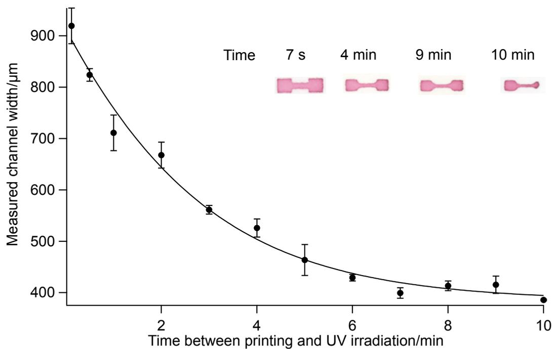
**Figure S-1.** Measurement of channel width in dependence of the time passed between printing and initializing UV curing (error bars: standard deviation for 3 patterns; the width of each single channel was measured at 6 positions and the mean value plotted as the channel width).
