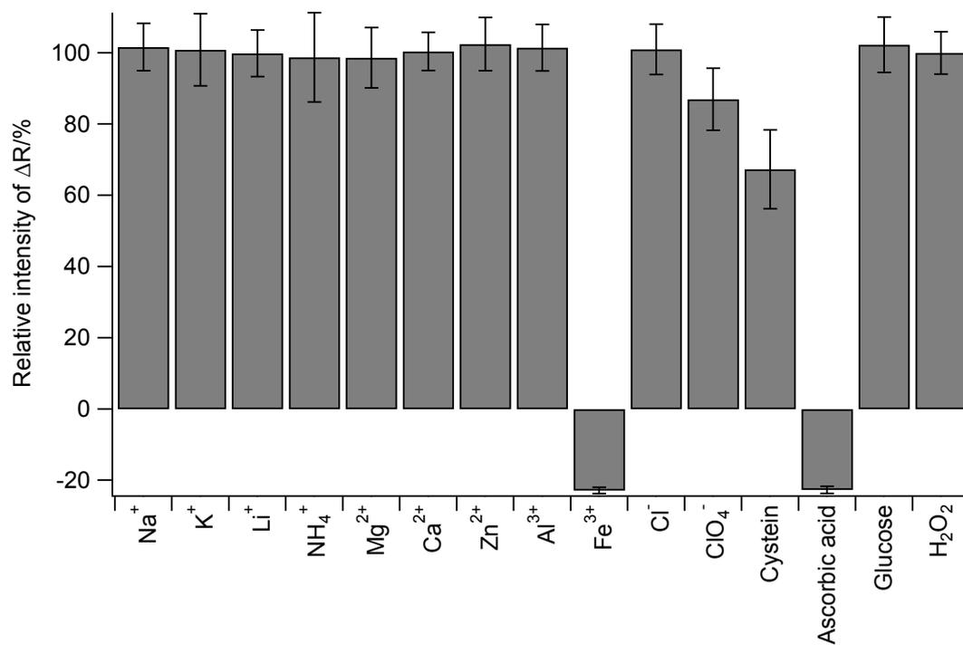
**Figure S-4.** Normalized colourimetric signal induced by the application of 0.5 mM  $\text{H}_2\text{O}_2$  solution in the presence of 1.0 mM of various foreign species (error bars: n=5). All cations have been applied as nitrate salts.
