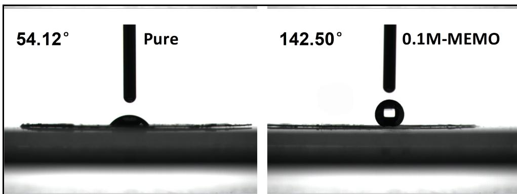
Fig. S5 Water contact angles for Non, 0.1M-MEMO modified  $\text{Fe}_2\text{O}_3@\text{SiO}_2$  NPs
