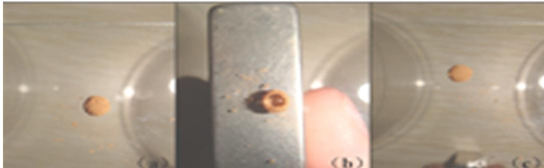
Fig.S6 Process of magnetic liquid marbles opened and closed reversibly under the action of a magnetic field.
