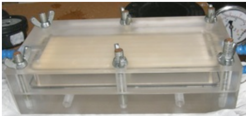
Figure S3: The membrane cell used for the experimental test.
