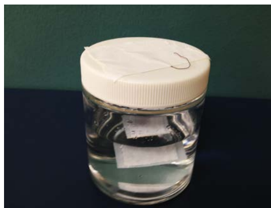
Figure S2: A) Cotton swatch glued to cover slip (front view). A copper wire is taped to the back of the cover slip. The jar contains the ZnO growth solution and the lid has a small hole for suspending the swatch by the wire. B) Cotton swatch glued to cover slip with copper wire taped to back of cover slip (tape: PELCO Tabs, 9 mm OD, Ted Pella Inc.) (rear view). C) Cotton fabric (supported on cover slip) suspended in ZnO growth solution. D) Top view of swatch suspended in ZnO growth solution. The copper wire was secured to the lid with label tape (Fisher Scientific) before incubating at 95 °C in an oven.
