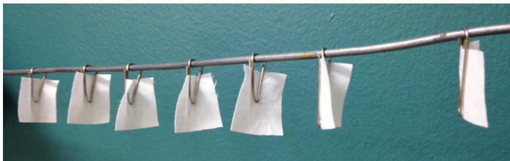
Figure S1: Cotton swatches after dip-coating in ZnO seed solution. The drying rack was mounted directly in an oven and cured at 120 °C for 1 hour.
