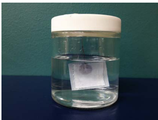
Figure S2: A) Cotton swatch glued to cover slip (front view). A copper wire is taped to the back of the cover slip. The jar contains the ZnO growth solution and the lid has a small hole for suspending the swatch by the wire. B) Cotton swatch glued to cover slip with copper wire taped to back of cover slip (tape: PELCO Tabs, 9 mm OD, Ted Pella Inc.) (rear view). C) Cotton fabric (supported on cover slip) suspended in ZnO growth solution. D) Top view of swatch suspended in ZnO growth solution. The copper wire was secured to the lid with label tape (Fisher Scientific) before incubating at 95 °C in an oven.
