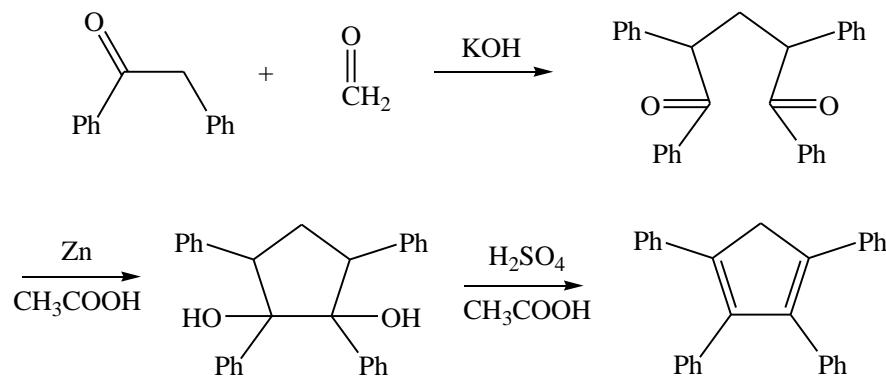
1,2,3,4,5-pentaphenyl cyclopentadiene was synthesized according reported strategy as below and the structure is checked according with reference (L. D. Field, K. M .Ho, C. M. Lindall, *Austr. J. Chem.*, 1990, **43**(2), 281-291.):
