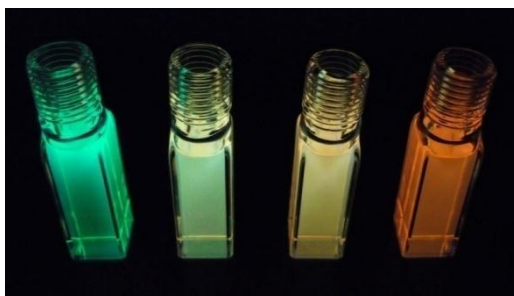
Figure S7. Visual fluorescence color changes of sensor 1b in the solution with various pH values (from left to right: 7.0, 5.2, 3.9, 2.8), the photo was taken under illumination of a handheld UV lamp.
