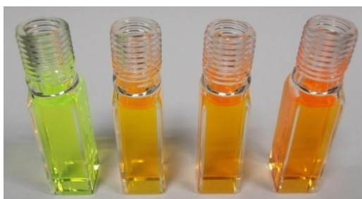
Figure S9. Visual color changes of sensor 1b in the solution with various pH values (from left to right: 7.0, 5.2, 3.9, 2.8).
