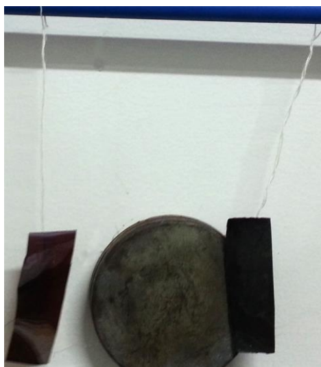
Figure S2 photograph shows that PI/ \alpha -Fe 2 O 3 (left) can not, but PI/Fe 3 O 4 (right) composite films can be attracted by a permanent magnet. The composite films are hung freely under an iron support with a permanent magnet in the middle.
