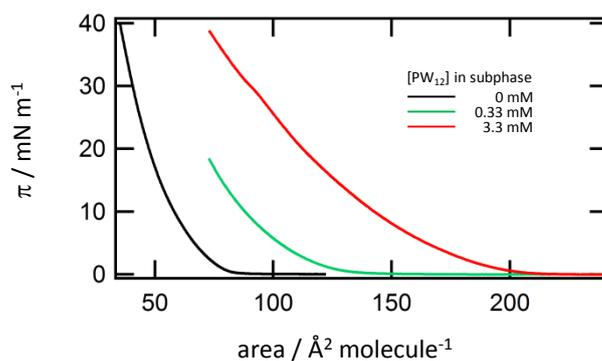
Figure S1.  $\pi$ -A isotherms for egg-PC monolayer at 22°C on Tris/HCl subphase containing different concentrations of PW<sub>12</sub>.
