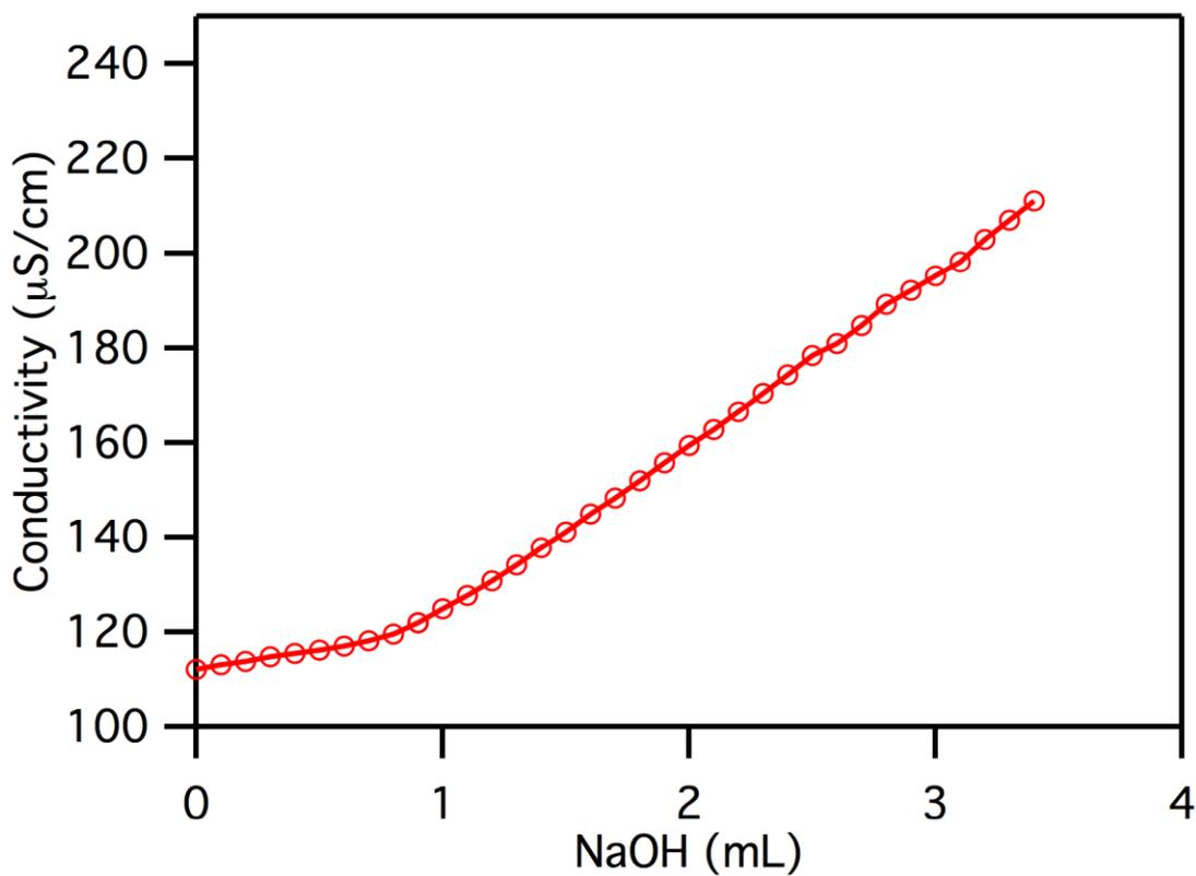
Figure S1. Conductometric titration curve of TEMPO oxidized cellulose at 5 mmol NaClO/g of cellulose without adding HCl.
