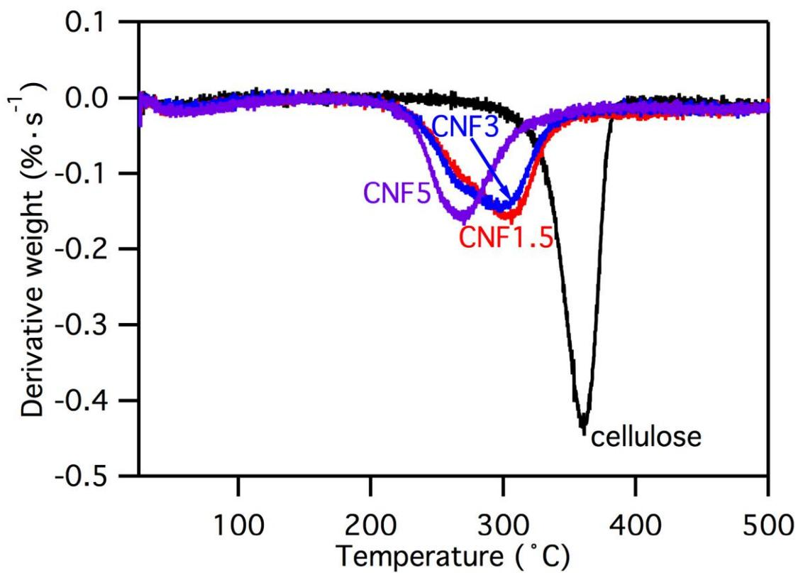
Figure S5. DTG curves of rice straw cellulose (black) and freeze-dried TEMPO oxidized and defibrillated CNF1.5 (red), CNF3 (blue) and CNF5 (purple).
