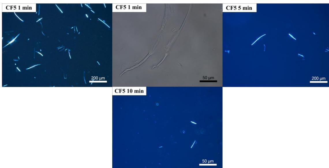
Figure S4. Optical microscopic images under cross polarizer of the precipitates from CF5 after various blending times
