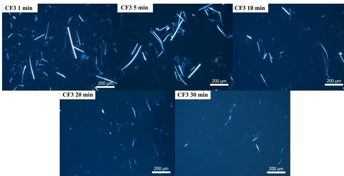
Figure S3. Optical microscopic images under cross polarizer of the precipitates from CF3 after various blending times
