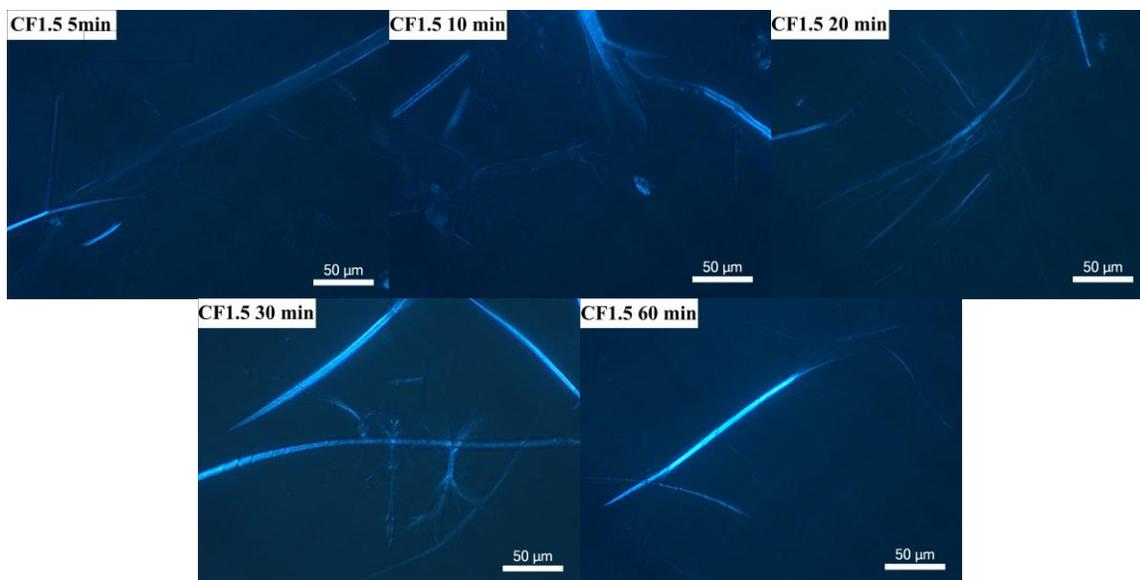
Figure S2. Optical microscopic images under cross polarizer of the precipitates from CF1.5 after various blending times
