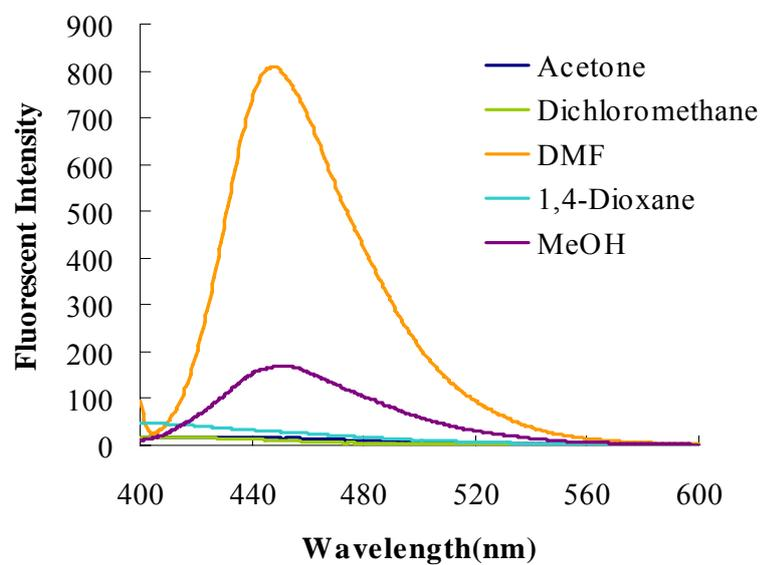
**Fig. S5** Fluorescence emission spectra of compound **2f** in organic solvents ( $\lambda_{\text{ex}}=325\text{nm}$ ).
