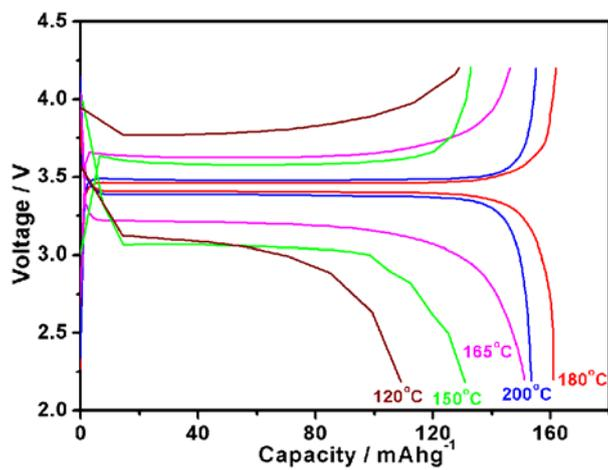
**Fig. S5** Initial charge and discharge curves of samples prepared at different time ( then calcined at 750 °C for 1 h ) at the current density of 0.1C in the potential range from 2.2 to 4.2 V.
