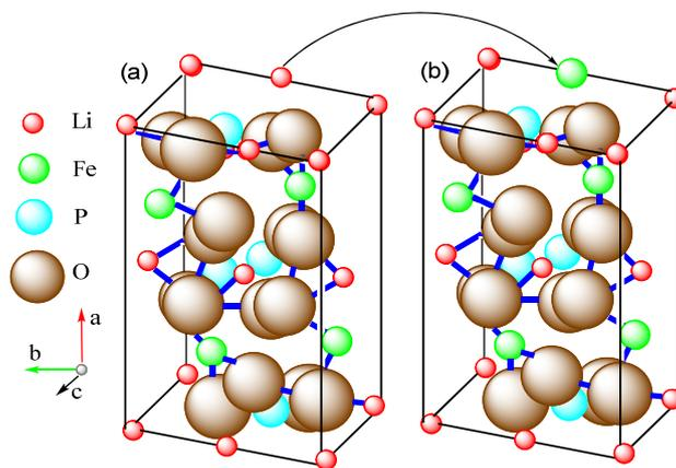
**Fig. S3** (a) and (c) Curved pathway for Li ion motion; (b) the blocked tunnel absence of Fe on Li sites
