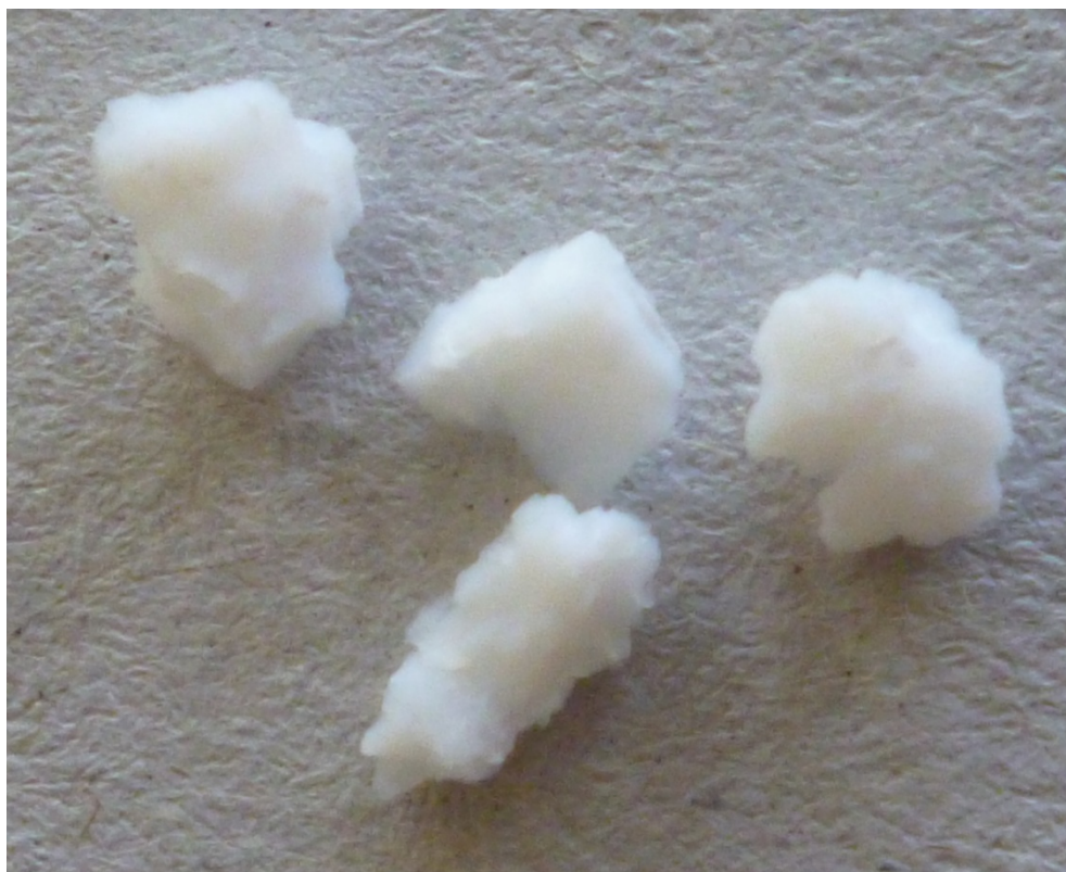
Fig. S17. Photo of silica aerogel HS_97 after supercritical drying
