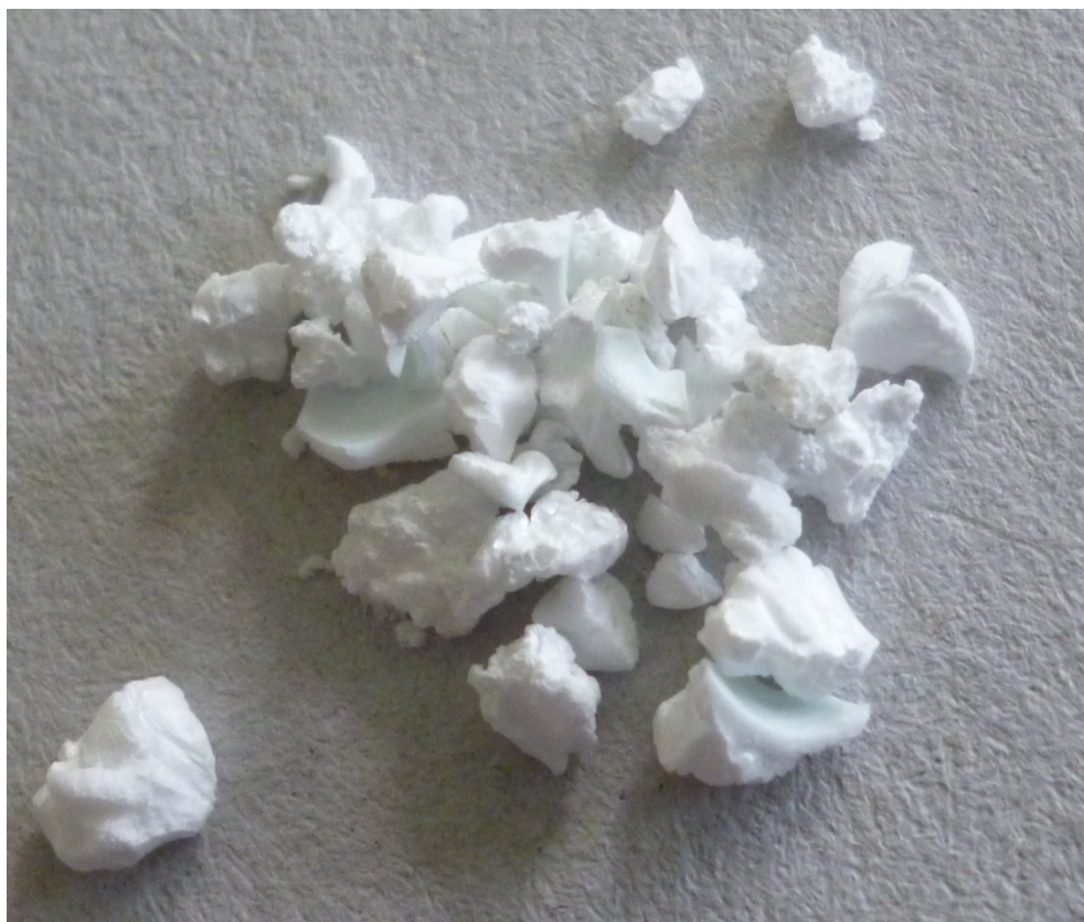
Fig. S22. Photo of zirconia aerogel HS_3.1 after supercritical drying
