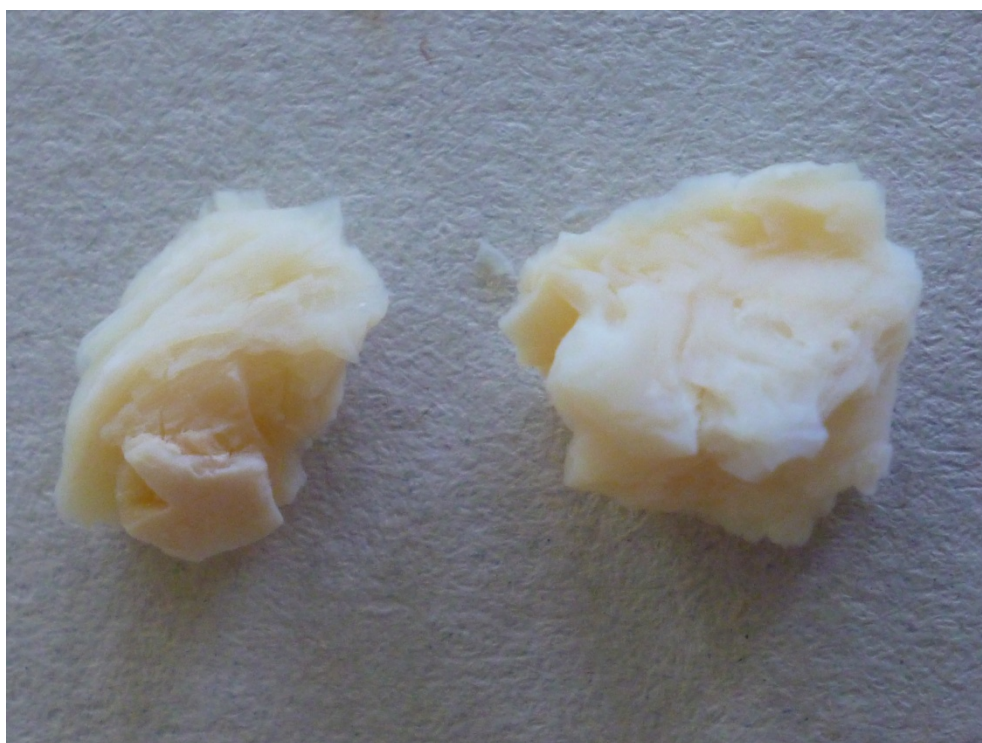
Fig. S18. Photo of silica aerogel HS_128 after supercritical drying
