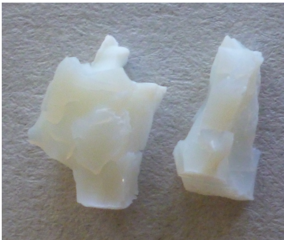
Fig. S16. Photo of silica aerogel HS_8 after supercritical drying
