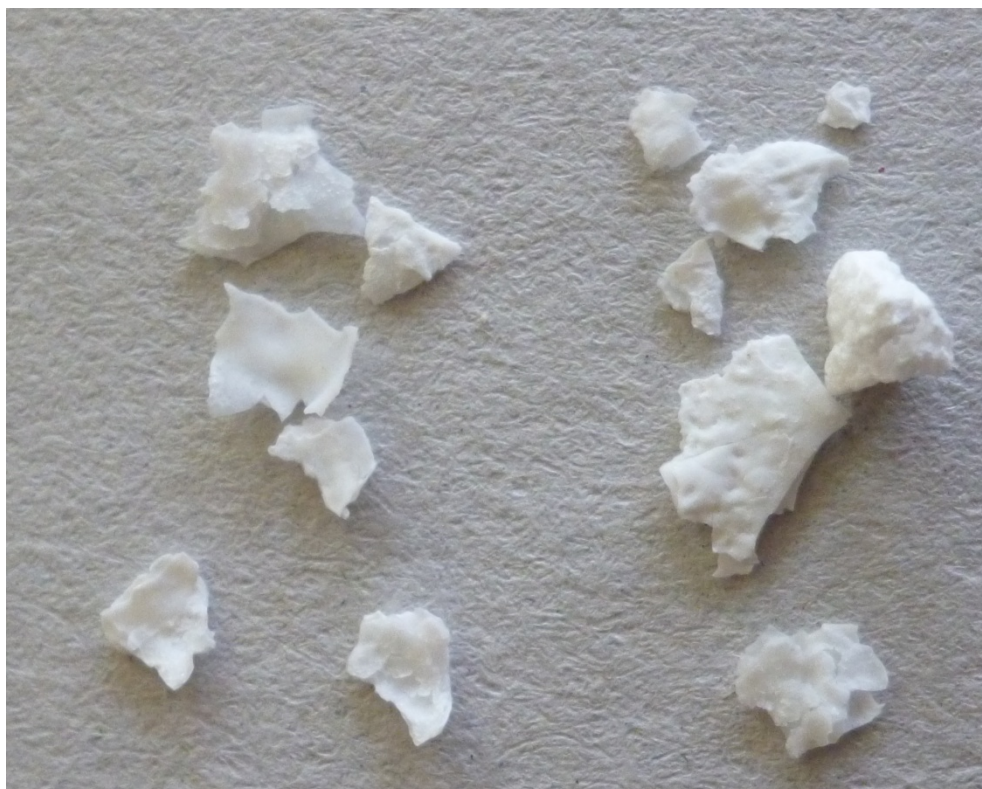
Fig. S15. Photo of silica aerogel HS_16.2 after supercritical drying
