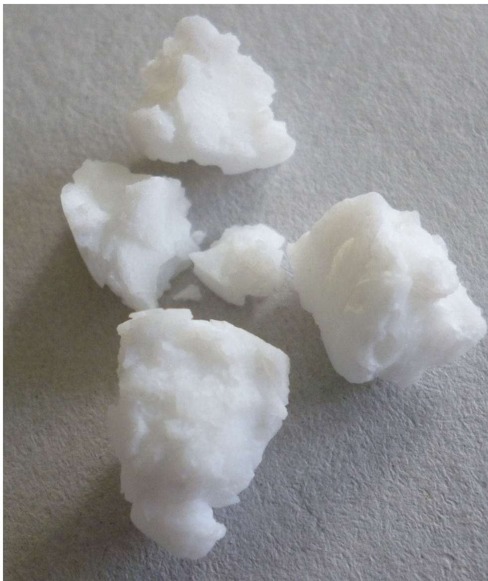
Fig. S19. Photo of silica aerogel HS_138 after supercritical drying
