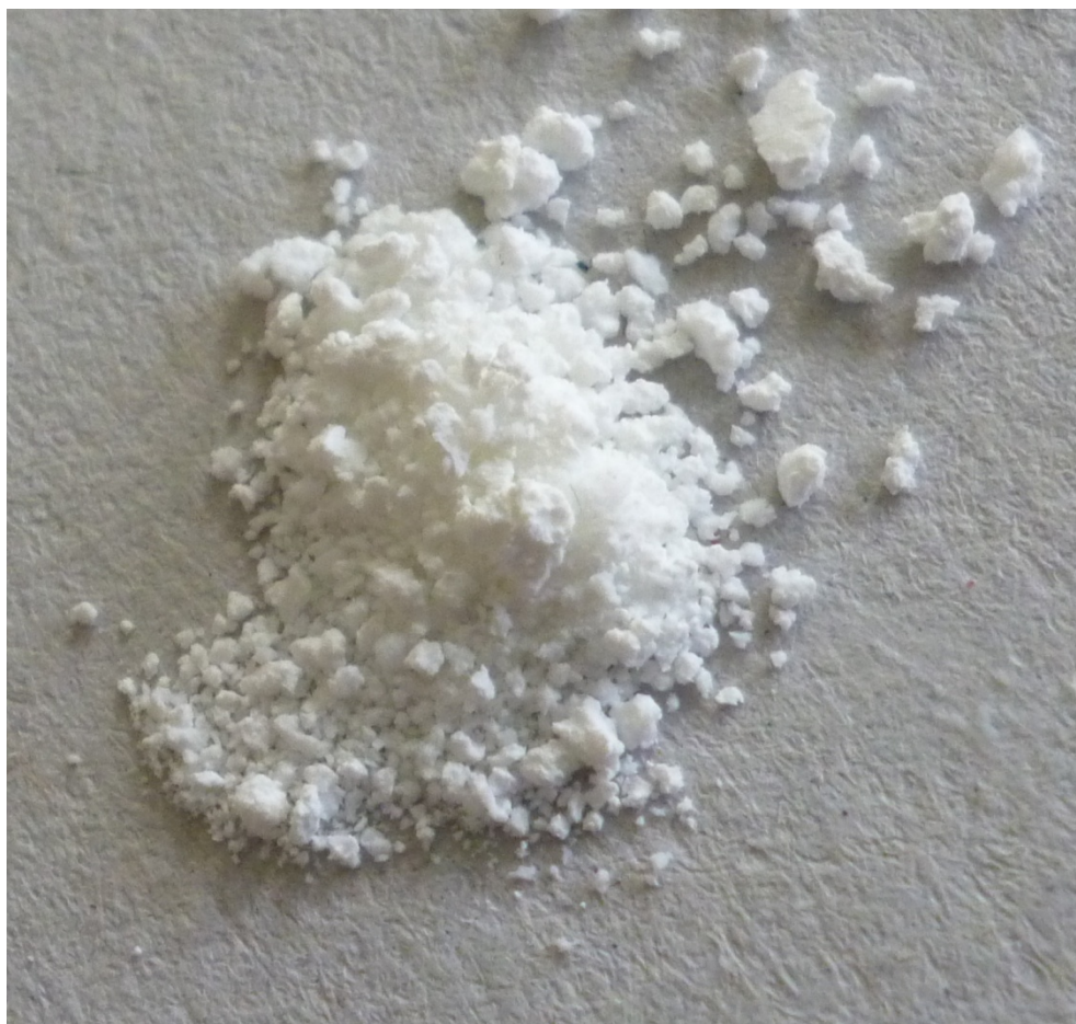
Fig. S27. Photo of silica/titania aerogel HS_115 after supercritical drying
