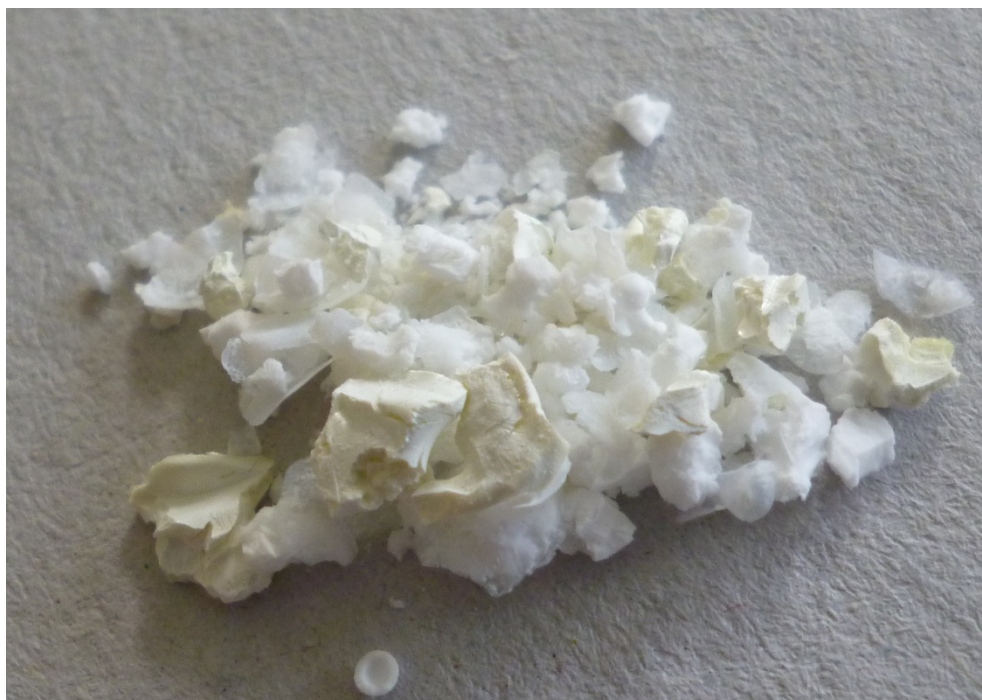
Fig. S23. Photo of zirconia aerogel HS_3.2 after supercritical drying
