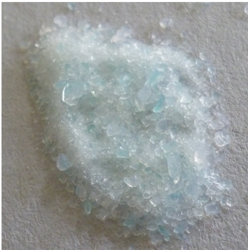
Fig. S24. Photo of zirconia aerogel HS_33 after supercritical drying
