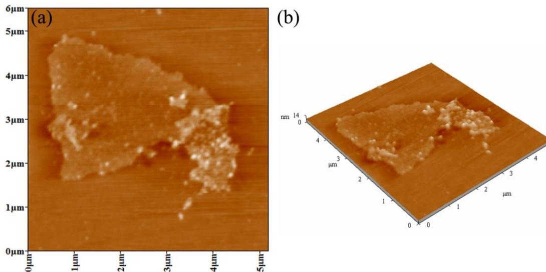
**Figure 4S.** AFM image of (a) GO–AEPTMS/SO<sub>3</sub>H, and (b) corresponding 3D image.
