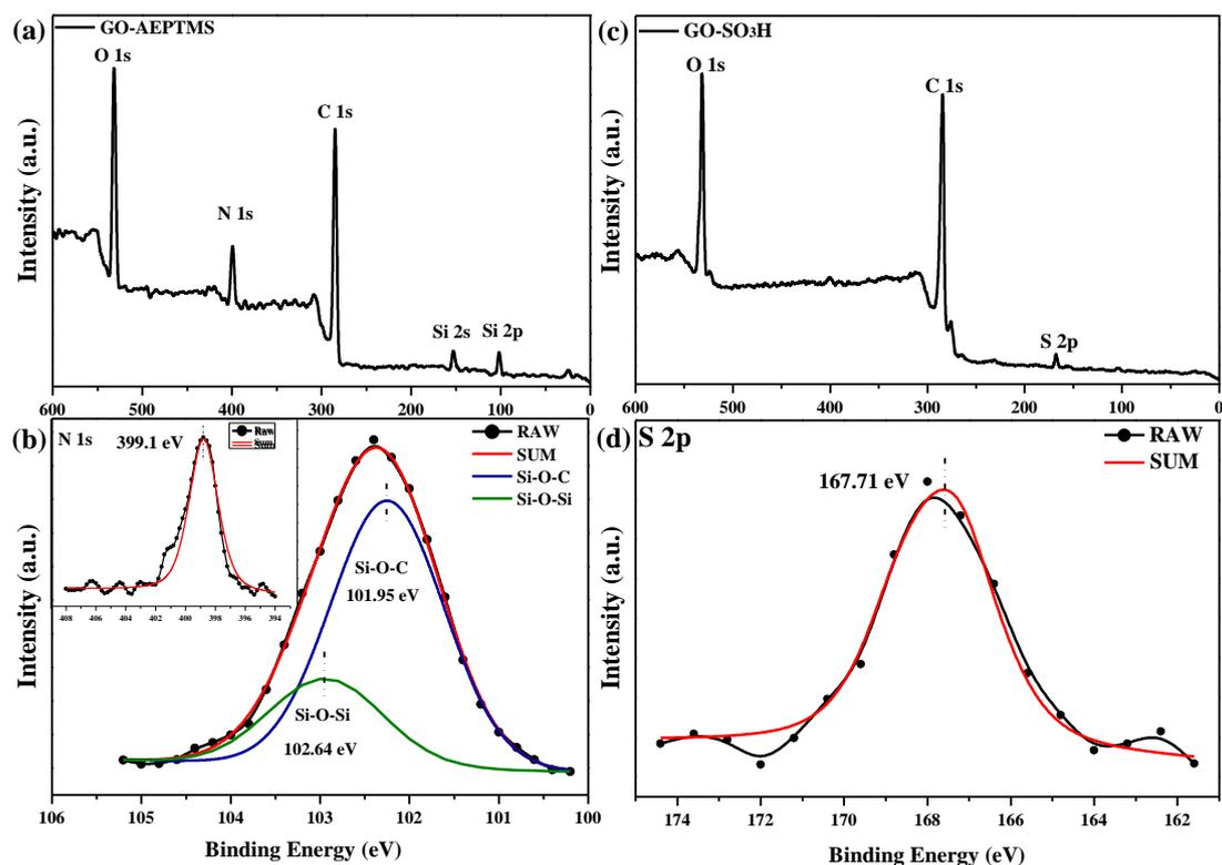
**Figure 2S.** (a) Full range, (b) Si 2p and (insert) N 1s XPS spectra of GO-AEPTMS hybrids, as well as (c) full range and (d) S 2p XPS spectra of GO-SO<sub>3</sub>H hybrids. The peak area ratio of Si-O-C in Si 2p of GO-AEPTMS is 75.7 %.
