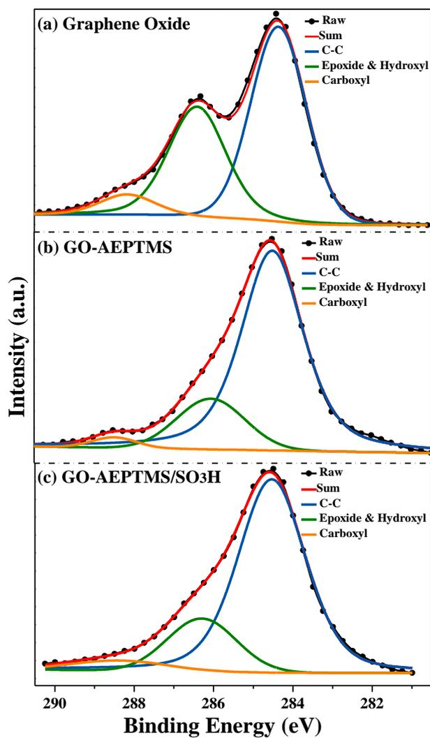
**Figure 1S.** C 1s XPS spectra of (a) GO (b) GO-AEPTMS hybrids and (c) GO-AEPTMS/SO<sub>3</sub>H hybrids, respectively.
