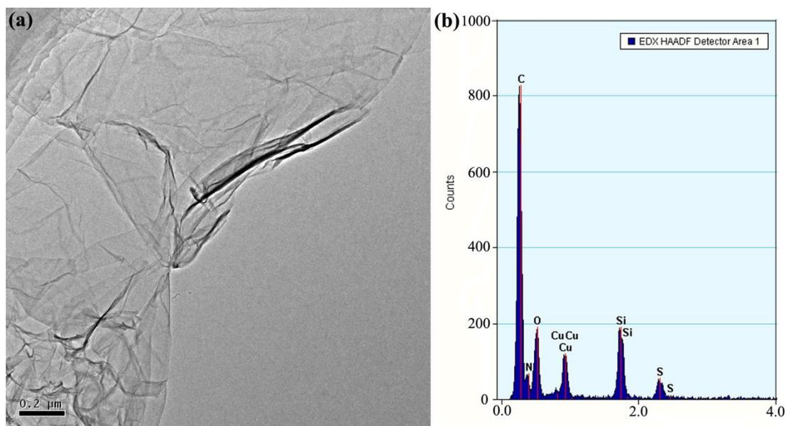
**Figure 3S.** (a) Typical TEM image of GO-AEPTMS/SO<sub>3</sub>H hybrids, and (b) corresponding EDX result.
