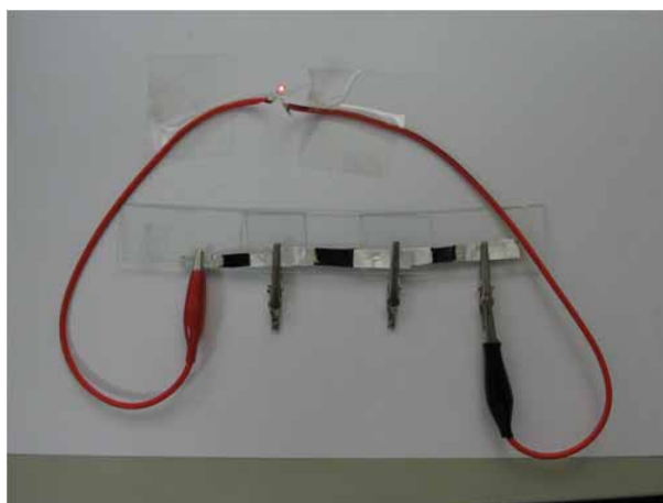
Fig.S14 Three A-SCs connected in series can illumine a LED light
