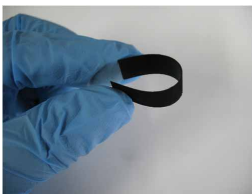
Fig.S10 Demonstration of the flexibility of CNFs/ MWCNTs (50%) aerogel film
