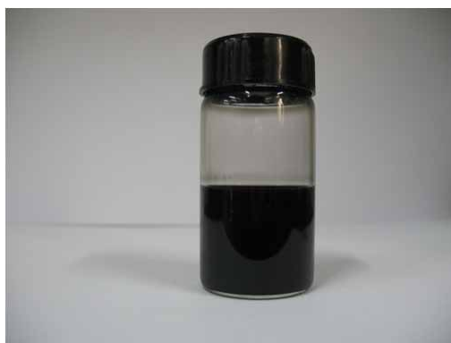
Fig.S4 Optical images of the aqueous dispersion of CNFs/MWCNTs (50%) suspension
