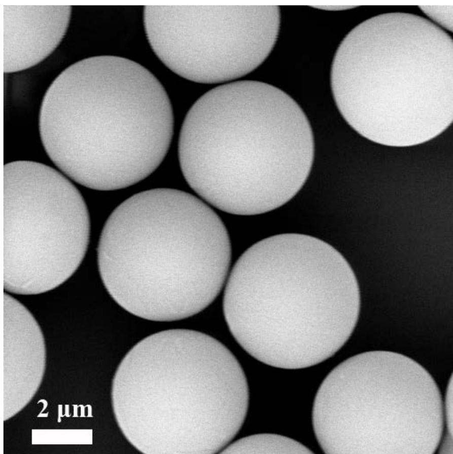
**Figure S5.** SEM image of the MF microspheres; Melamine 0.625g, formaldehyde 0.9 g, formic acid 7  $\mu$ L, reaction temperature 70  $^{\circ}$ C, and reaction time 2 h.
