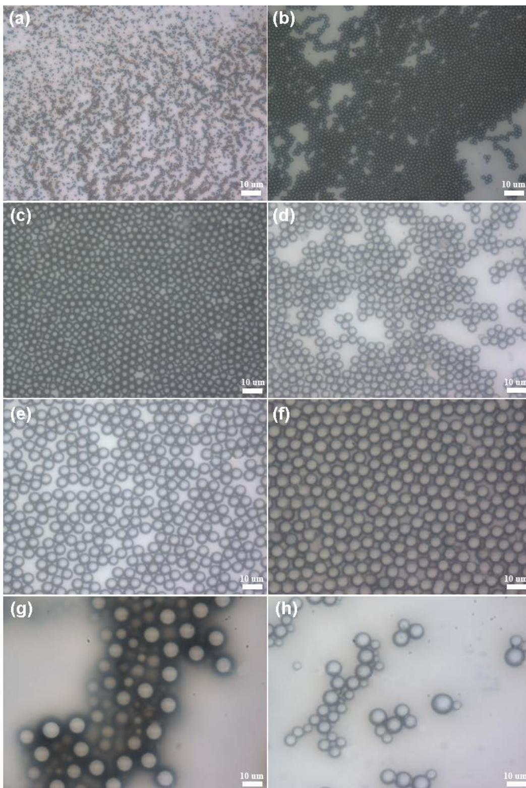
**Figure S3.** Optical images of the effect of formic acid amount on size of the MF microspheres:
