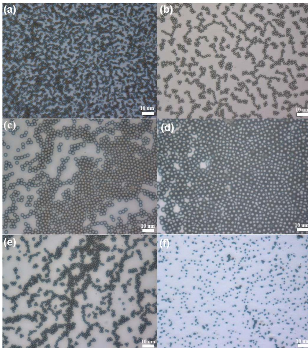
**Figure S2.** Optical images of the effect of reaction temperature on size of the MF microspheres:
