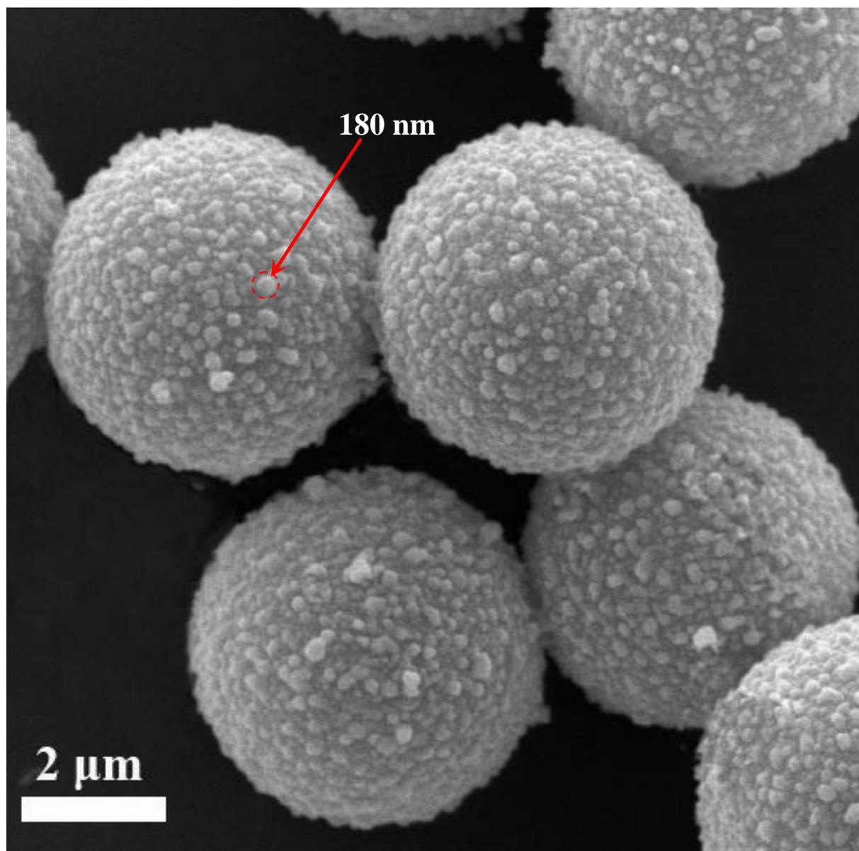
**Figure S6.** SEM image of the MF/Ag-NPs microspheres synthesized with 10:1 mass ratio of  $\text{AgNO}_3$  to MF microspheres.
