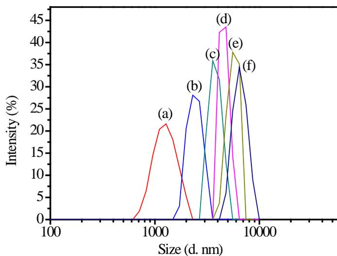
**Figure S4.** Hydrodynamic diameter distribution of the MF microspheres synthesized with different dosages of formic acid: (a) 50 $\mu$ L, (b) 25  $\mu$ L, (c) 10  $\mu$ L, (d) 7  $\mu$ L, (e) 5  $\mu$ L, (f) 4  $\mu$ L; Melamine 0.625g, formaldehyde 0.9 g, temperature 70  $^{\circ}$ C, reaction time 2 h.
