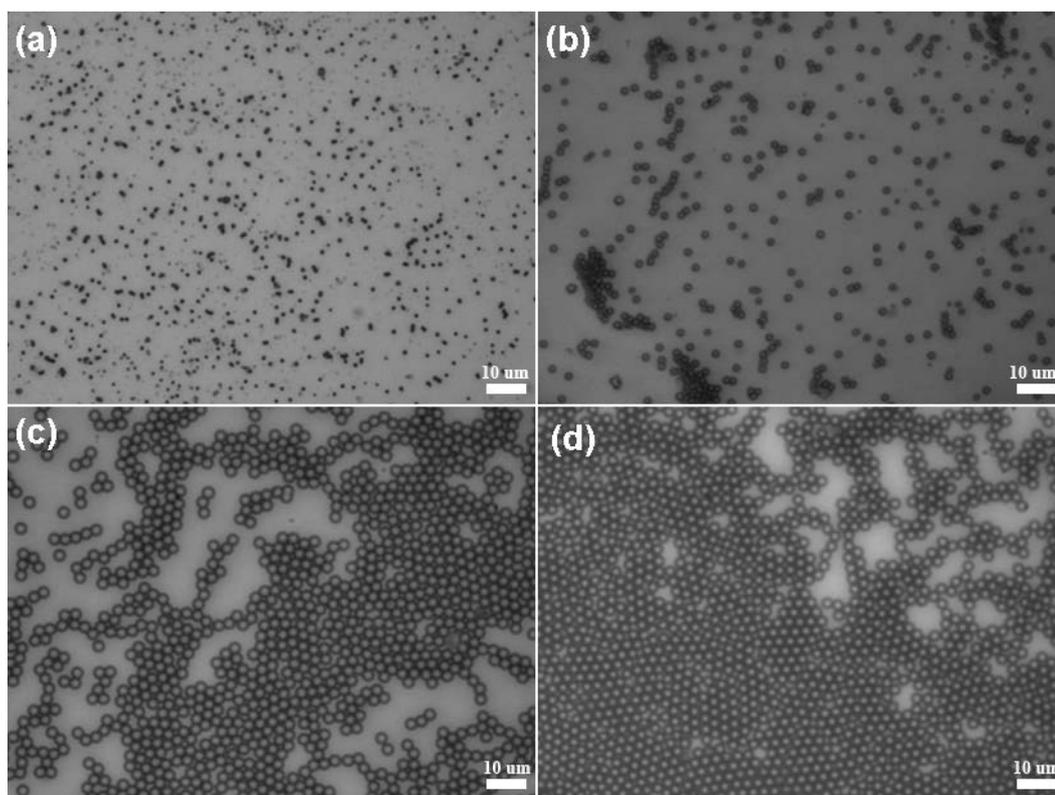
**Figure S1.** Optical images of the effect of reaction time on size of the MF microspheres: (a) 0.5 h, (b) 1.0 h, (c) 2.0 h, (d) 3.0 h; Melamine 0.625g, formaldehyde 0.9 g, temperature 60 °C, formic acid 10  $\mu$ L.
