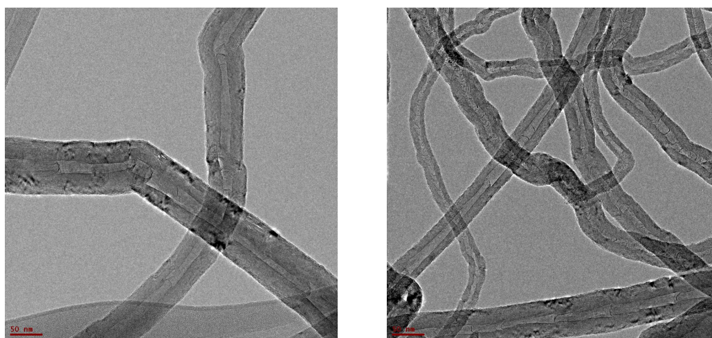
Fig. S11 TEM images of Pd/CFCNT50 (left) and Pd/CFCNT50 (right) produced with the reaction time of 24 hour.
