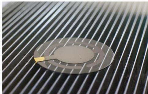
**Figure S2.** (A) Electrode mass change and the total charge passed during cathodic deposition of a ~100 ML Te film and (B) a photographic image of the resulting sample (a quartz crystal with Au electrodes; the WE-side is coated with a thin film of Te).
