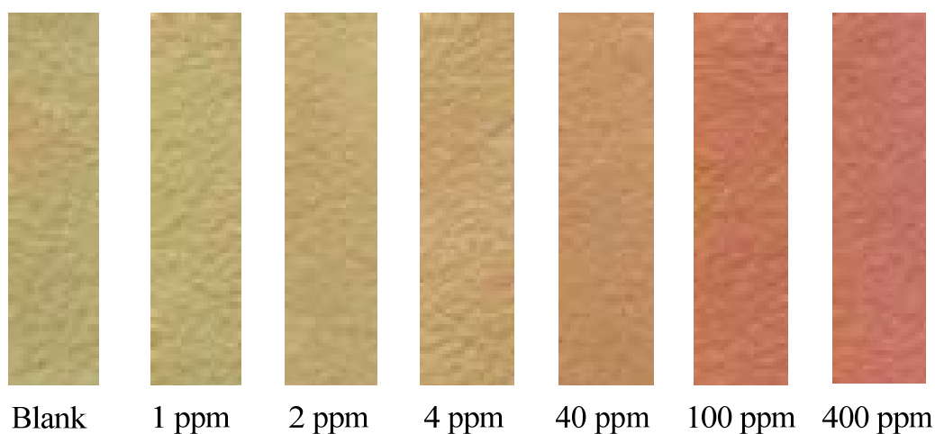
Fig. S7 Colour changes of test paper containing chemodosimeter 1 with different concentration of F^- in water.
