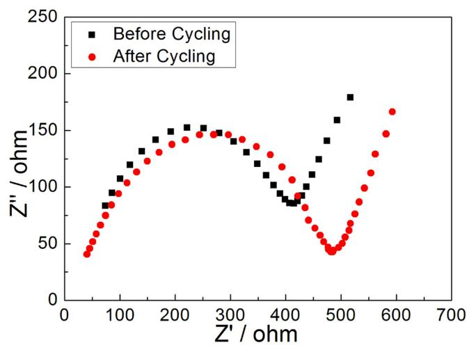
**Fig. S6** Electrochemical impedance spectroscopy (EIS) curves of the  $\text{Mn}_2\text{O}_3$  electrode.
