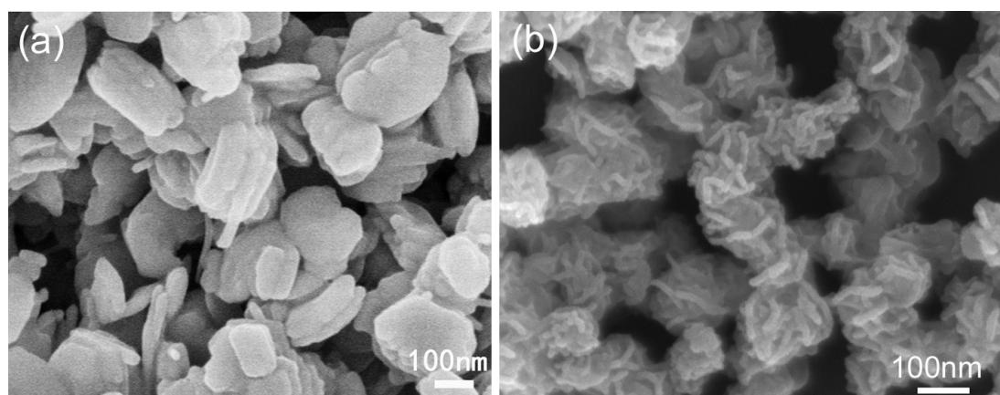
**Fig. S2** SEM images of as-prepared MnO<sub>2</sub> (a) without the addition of P123, (b) without the addition of CNTs.
