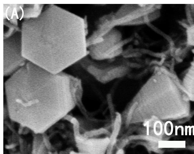
**Fig. S3** SEM image of MnO<sub>2</sub> nanocones/CNTs composite grown at different reaction times of 2 h at 120 °C.
