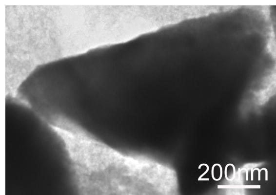
**Fig. S5** SEM image of the as-prepared  $\text{Mn}_2\text{O}_3$  after cycles.
