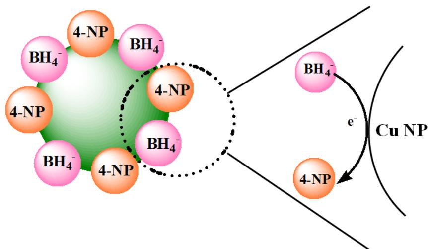
Fig. S4: Schematic representation of catalytic process occurring on Cu nanoparticles embedded in TOCNF film.
