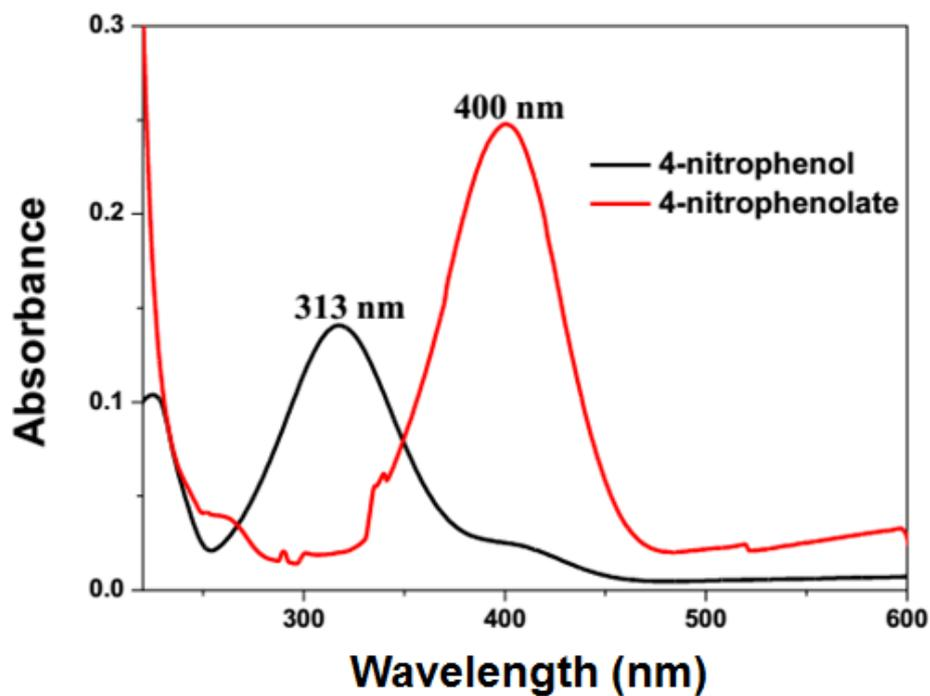
Fig. S2: UV-Vis spectra of 4-nitrophenol and 4-nitrophenolate ion.
