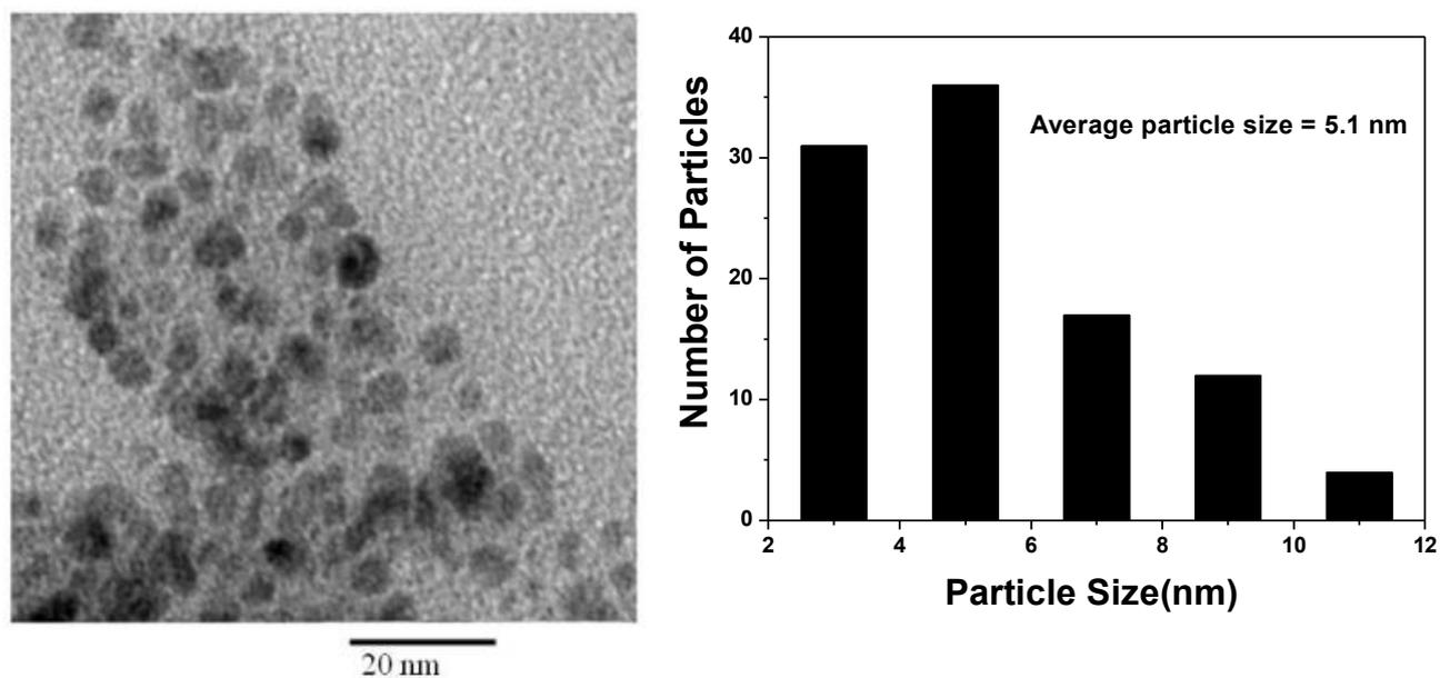
Fig. S1: (Left) A TEM image of Cu nanoparticles prepared using ascorbic acid as a reducing agent and (right) a histogram of particle size distribution.
