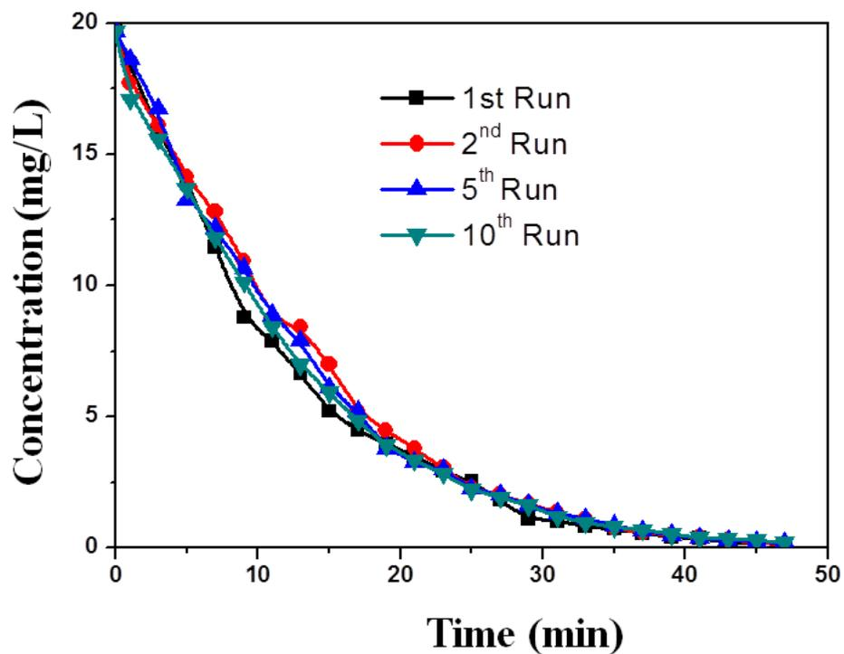
Fig. S3: Plot of concentration versus time of 4-nitrophenol reduction for multiple runs (1, 2, 5, 10) on the same Cu-TOCNF film.
