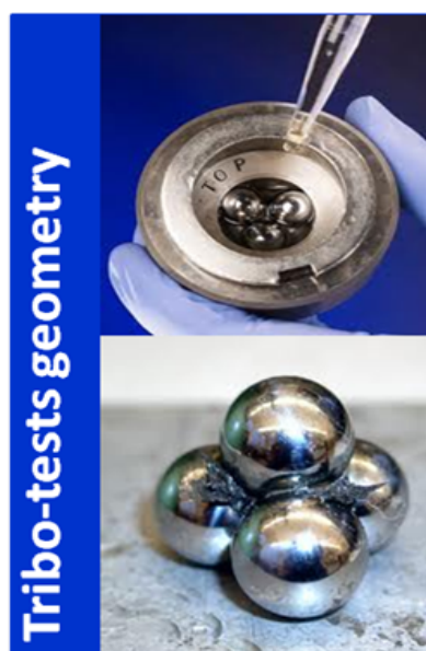
Figure S1: Pictorial view of four balls arrangement during the tribo-test.
