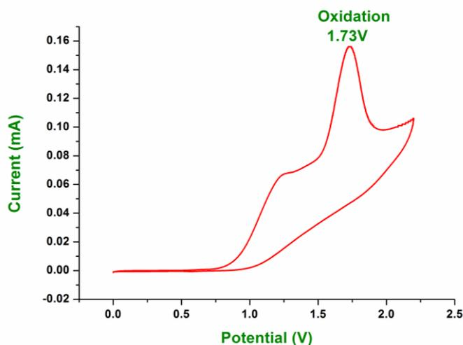
**Fig. S12** Cyclic voltammogram of **3** (0.5 mM) in mixed solutions ( $\text{CHCl}_3/\text{CH}_3\text{CN} = 5:1$ , v/v, containing 0.1 M  $\text{TBAClO}_4$ ) at a scan rate of 5 mV/s using tin doped indium oxide as working electrode.
