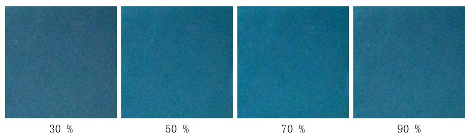
**Fig. S6** The optical images of the blue  $\text{PSVP}(\text{PDA})_{0.12}$  fibre mats under variations of relative humidity.
