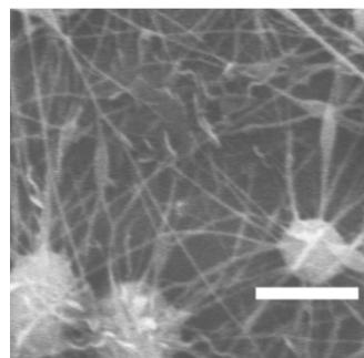
**Fig. S1** SEM image of  $\text{PSVP}(\text{DA})_{0.12}$  supramolecular electrospun fibres with  $50 \text{ mg mL}^{-1}$  PS-*co*-P4VP in the precursor. The scale bar is  $5 \mu\text{m}$ .
