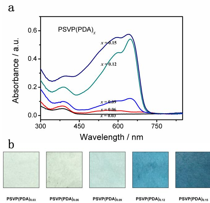
**Fig. S2** (a) DRUVS and (b) optical images of  $\text{PSVP}(\text{PDA})_x$  fibre mats obtained by photopolymerization.
