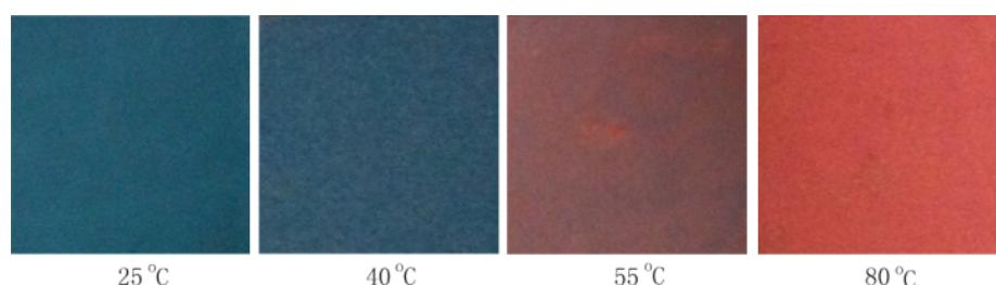
**Fig. S5** The optical images of the  $\text{PSVP}(\text{PDA})_{0.12}$  fibre mats after annealing at different temperatures.
