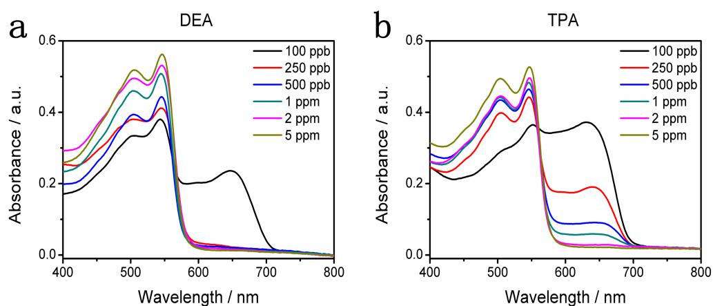
**Fig. S4** DRUVS of the PDA-embedded fibre mats after exposure to various concentrations of (a) DEA and (b) TPA vapour.
