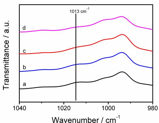
**Fig. S3** ATR FTIR spectra at range of 980–1040  $\text{cm}^{-1}$  of (a) PSVP(DA)<sub>0.12</sub>, (b) blue PSVP(PDA)<sub>0.12</sub> fibre, (c) red PSVP(PDA)<sub>0.12</sub> fibres obtained by thermal treatment and (d) red PSVP(PDA)<sub>0.12</sub> fibres obtained by exposure to 500 ppb TEA vapour.
