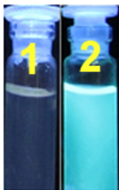
Fig. s7 Fluorescence colour of the probe in absence (1) and presence (2) of \text{Cr}^{3+} ion
