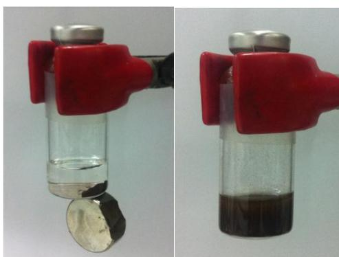
**Figure S1.** Magnetic separation of Pd-Fe<sub>3</sub>O<sub>4</sub> after the reaction.
