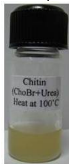
Fig. S4 . \alpha -Chitin (6% w/w) solubilized in choline chloride- urea 1: 2 employing different techniques as shown in Table 1
