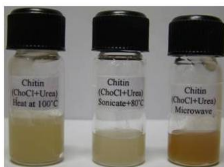
Fig. S4 . \alpha -Chitin (6% w/w) solubilized in choline chloride- urea 1: 2 employing different techniques as shown in Table 1
