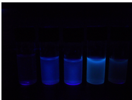
Figure S8. Photo images of TTZ-1 and TTZ-Pyr products dispersed in EtOAc under a handy UV light. From left to right are: TTZ-1, TTZ- Methylmethacrylate products, TTZ- Styrene products, TTZ- Ethene products and TTZ- Ethynyltrimethylsilane products.
