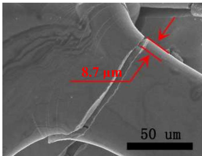
**Fig. S2.** The SEM image of the amorphous Ni-P alloy with the physical extrusion.
