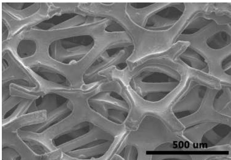
**Fig. S1.** SEM images of the pure nickel foam
