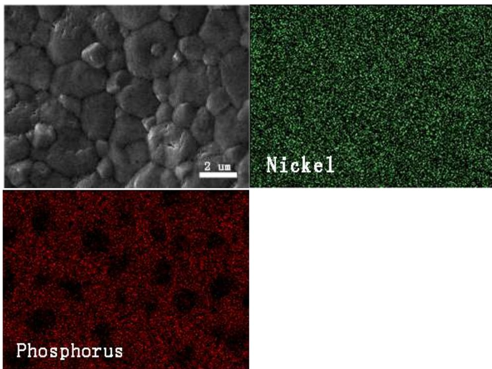
**Fig. S4.** The element mapping of crystal Ni-P alloy.
