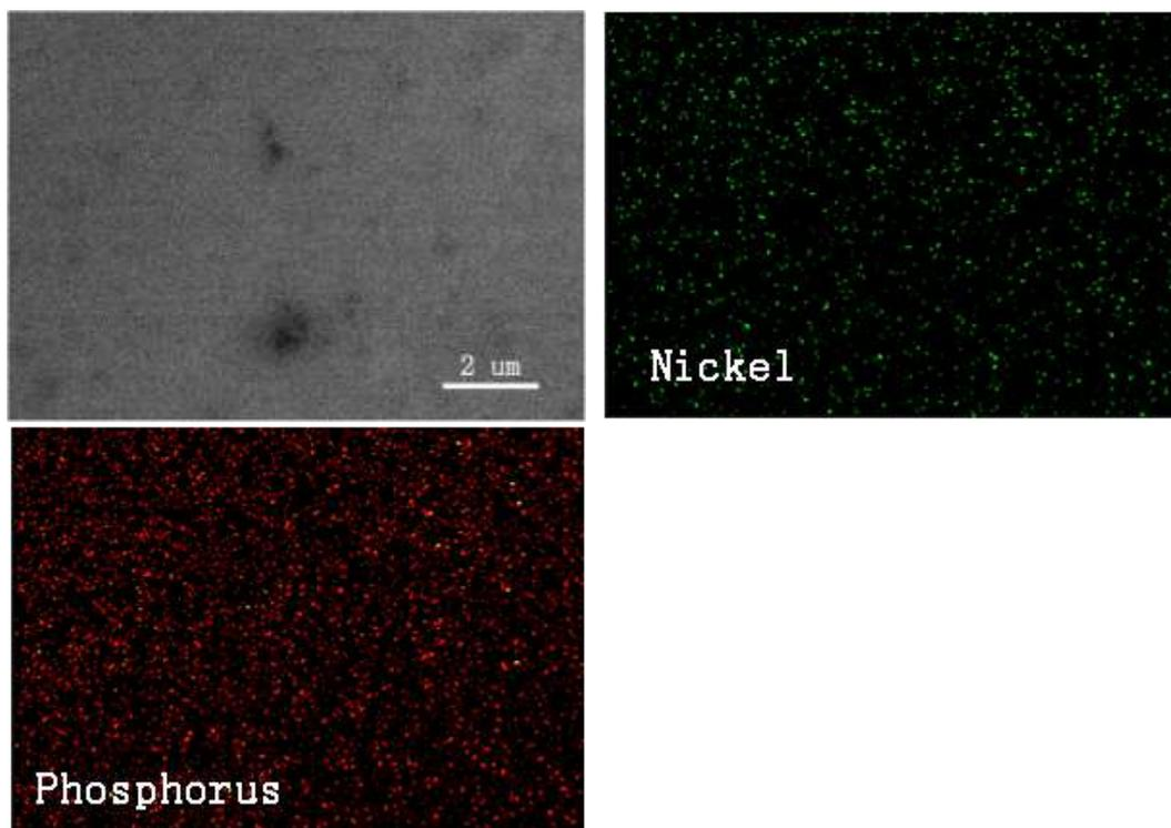
**Fig. S3.** The element mapping of amorphous Ni-P alloy.
