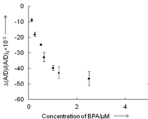
Figure S9. Binding isotherm of BPA in ethylacetate towards MIP-NPs in the presence of BPA-Au NPs. MIP-NPs: 0.22 mg/mL; BPA-Au NPs: 0.88 mg/mL Estimation of affinity constant of BPA to MIP-NPs in the presence of BPA-Au NPs by using the below equation.
