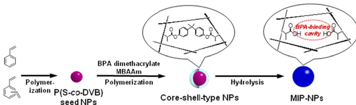
Figure S2. Schematic diagrams of the preparation of MIP-NPs for BPA by two-step emulsifier-free emulsion copolymerization
