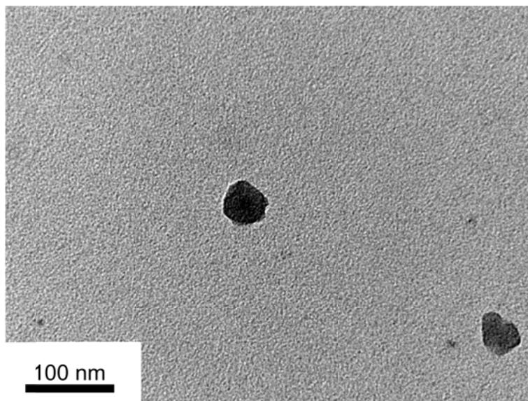
Figure S8. TEM photographs of NIP-NPs prepared by two-step emulsifier-free emulsion polymerization
