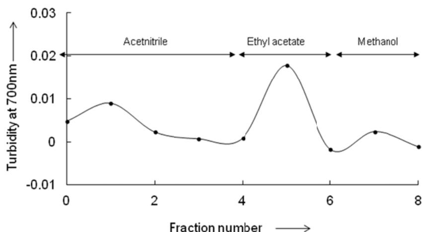
Figure S4. Elution profile of MIP-NPs in BPA-immobilized affinity chromatography with three different eluents (acetonitrile, ethylacetate and methanol). MIP-NPs elution was detected by turbidity at 700nm.
