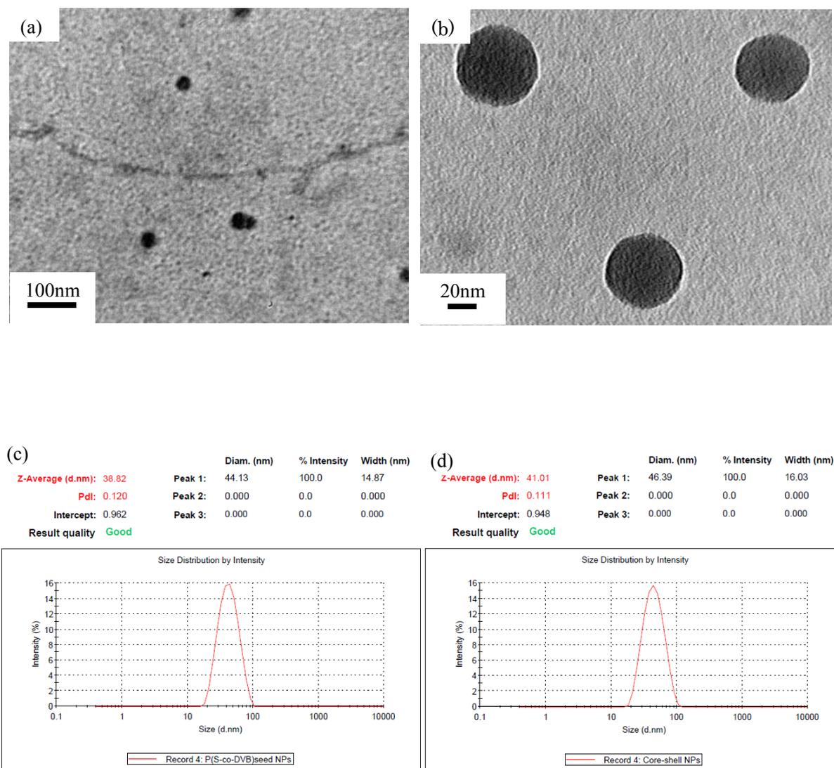
Figure S3. TEM images of P(S-co-DVB) seed NPs (a) and core-shell type NPs (b), and DLS data of P(S-co-DVB) seed NPs (c) and core-shell type NPs (d)
