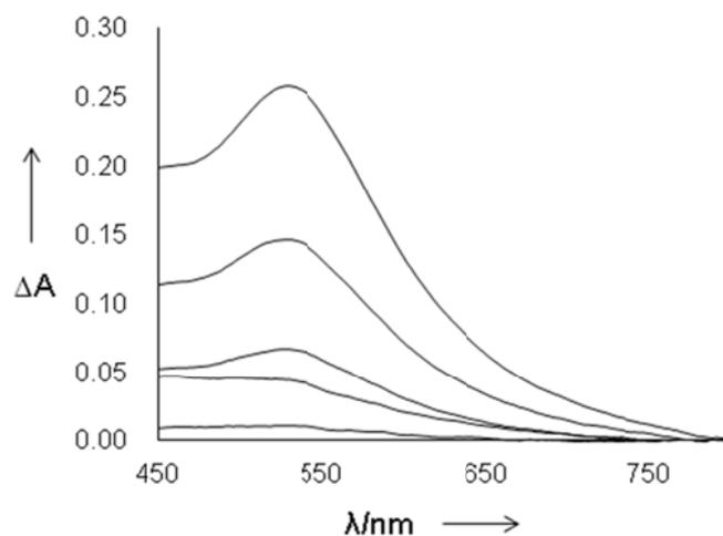
Figure S6. Effect of BPA-Au NPs concentrations on the change of BPA-Au NPs extinction. BPA-Au NPs concentration: 0.05, 0.10, 0.25, 0.50, 0.88 mg/mL, from bottom to top.
