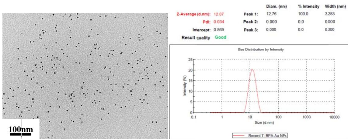
Figure S1. Synthesis scheme of BPA-thiol derivative (a) and TEM image of BPA-Au NPs (b) and DLS data of BPA-Au NPs (c)
