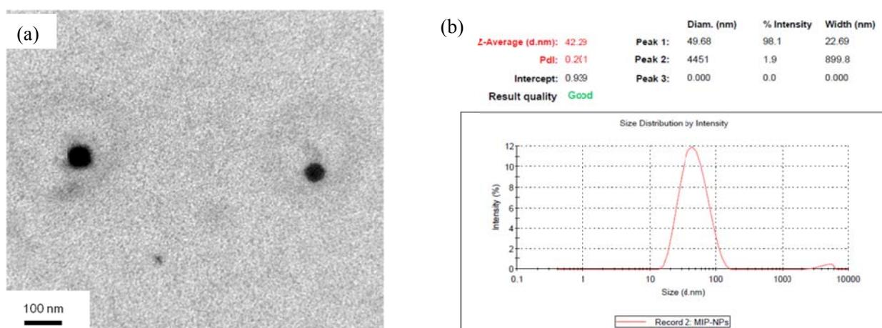
Figure S5. TEM image (a) and DLS data (b) of MIP-NPs in the fraction 5<sup>th</sup> from affinity chromatography utilizing BPA-immobilized silica gel
