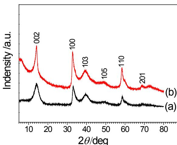
**Fig. S1** XRD patterns of (a) MoS<sub>2</sub>/GNS-S1 and (b) MoS<sub>2</sub>/GNS-S2 composites
