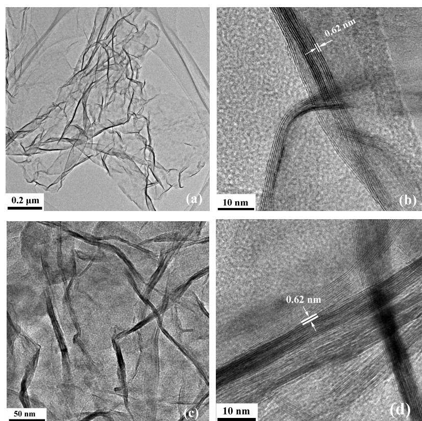
**Fig. S2** TEM/HRTEM images of (a, b) MoS<sub>2</sub>/GNS-S1 and (c, d) MoS<sub>2</sub>/GNS-S2 composites.
