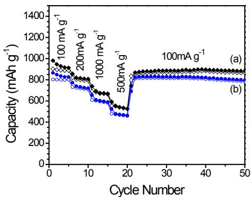
**Fig. S4** Rate capability of (a) MoS<sub>2</sub>/GNS-1 and (b) MoS<sub>2</sub>/GNS-2 composites at different charging/discharging current densities.
