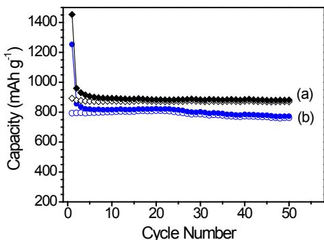
**Fig. S3** Cycling performances of (a) MoS<sub>2</sub>/GNS-1 and (b) MoS<sub>2</sub>/GNS-2 composites at a current density of 100 mA g<sup>-1</sup>.
