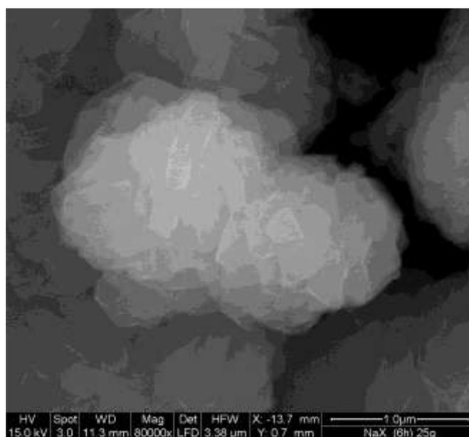
**Figure S2.** SEM images of the synthesized FAU nanocrystals i) at 6 hours of hydrothermal treatment.
