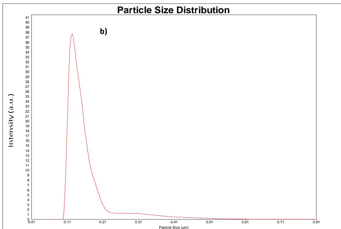
**Figure S3.** DLS distribution curves of the synthesized FAU nanocrystals i) (a) and ii)(b) obtained at 6 hours of reaction.
