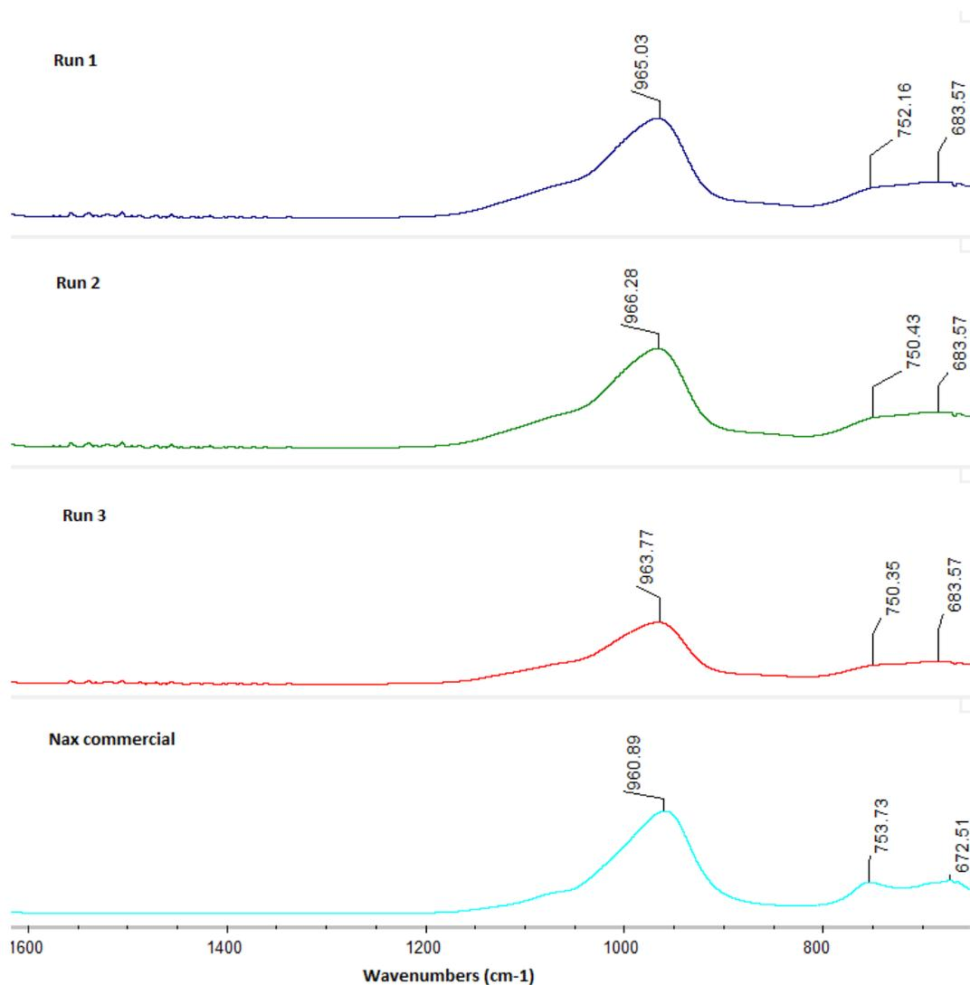
**Figure S4.** IR spectra collected on different samples (i. e. of different runs) of the synthesized FAU nanocrystals i) obtained at 6 hours of reaction. The IR spectrum obtained from the commercial NaX powder is showed for comparison.
