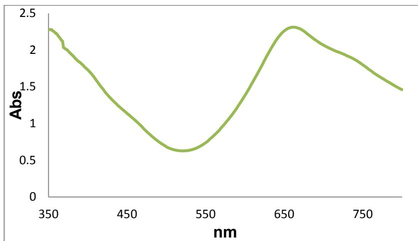
**Figure S11.** UV-visible spectra of a saturated solution of  $\text{ZnPc8SF}_{144}$  in  $\text{CCl}_4$ ;  $\lambda_{\text{max}}$  is at 664 nm, shoulder 721 nm. This shows substantial aggregation of the poorly soluble dye.
