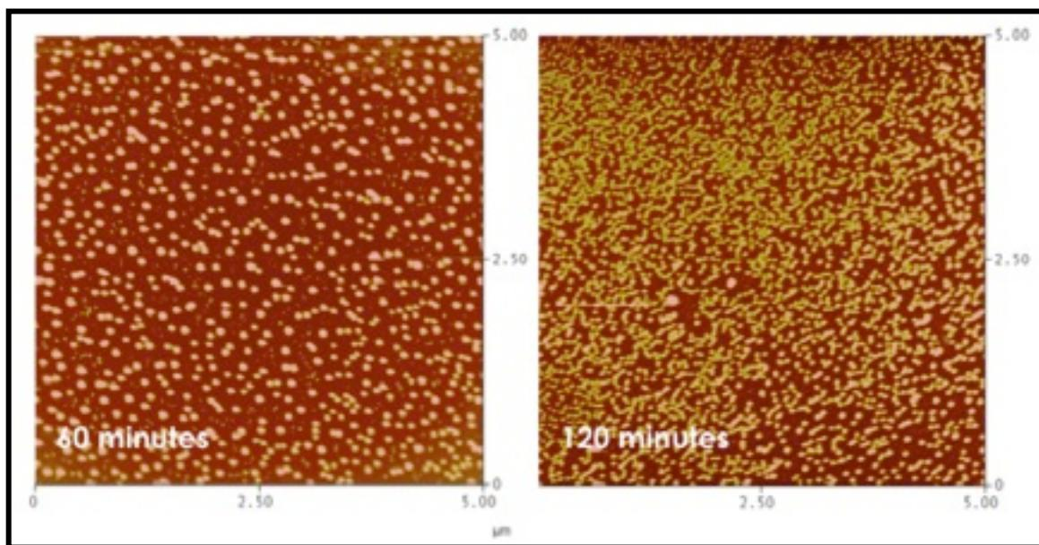
**Figure S9.** AFM images of nanoparticles formed from  $\text{Pc}16\text{S}/\text{C}_60$  ratio 1:15,  $[\text{Pc}] = 0.1 \text{ mM}$ , after 60 and 120 minutes of soaking in solution.
