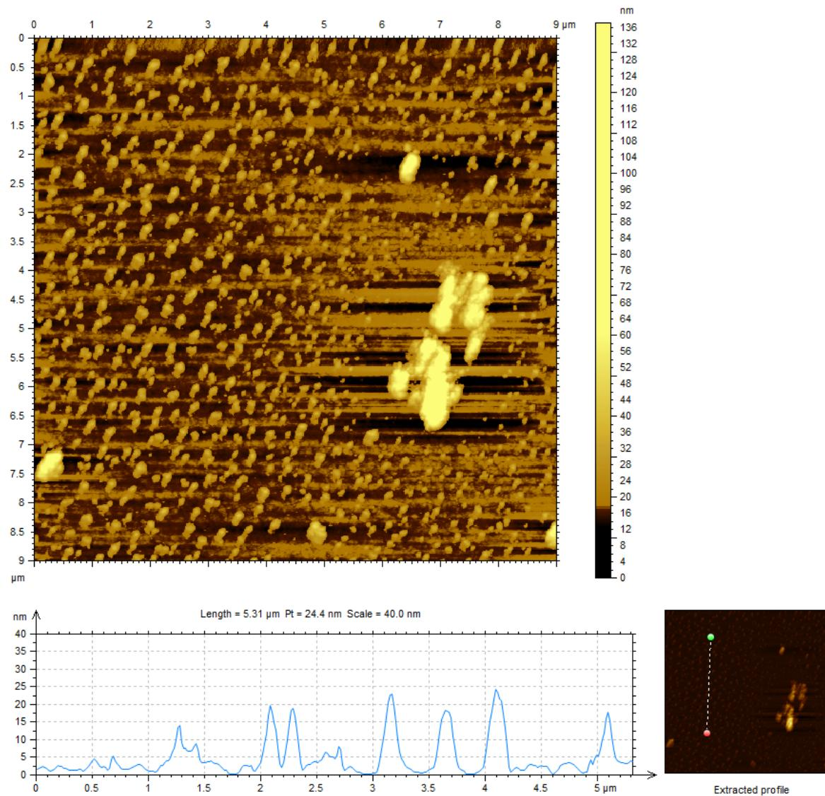
**Figure S5.** AFM image with height profile of aggregates formed from soaking the ITO slide in a 4.5 mM C<sub>60</sub> solution in toluene for 60 min.
