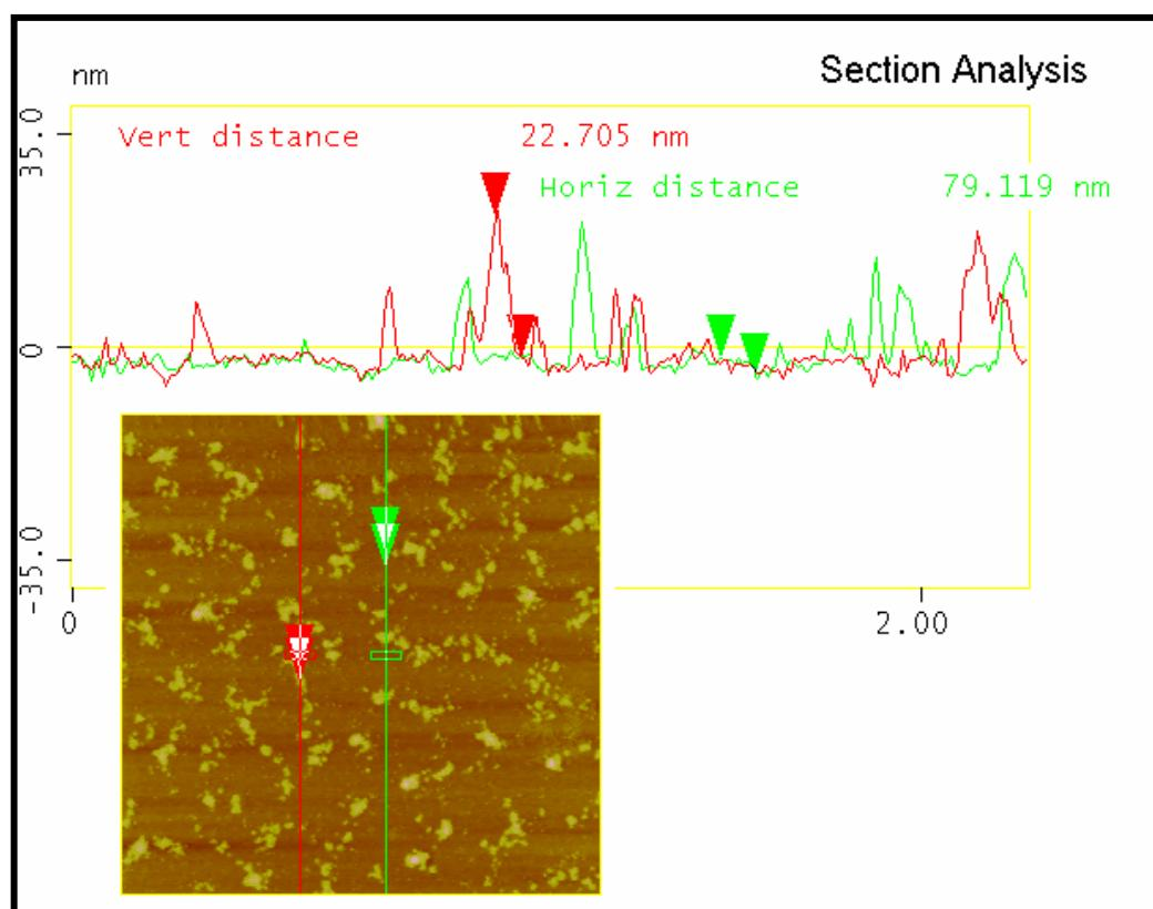
**Figure S4.** AFM image of the less uniform aggregates formed by dipping ITO slides into Pc8S solution.
