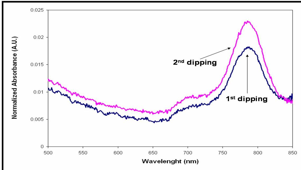
**Figure S6.** UV-Vis absorption spectra of Pc16S on ITO electrode after 1 and 2 immersions of 1 hour each in toluene solution of Pc16S (0.3 M). Absorption maxima correspond to the Q band of Pc16S.
