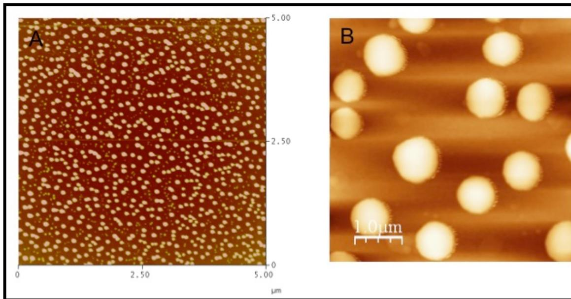
**Figure S8.** AFM images of nanoparticles formed from  $\text{Pc}16\text{S}/\text{C}_60$  in ratio 1:15 at different concentration of  $\text{Pc}$ : (A)  $[\text{Pc}] = 0.1 \text{ mM}$ , where the average nanoparticle height is 60 nm and width is 40 nm, (B)  $[\text{Pc}] = 0.3 \text{ mM}$ , average nanoparticle height 130 nm, average width 800 nm.
