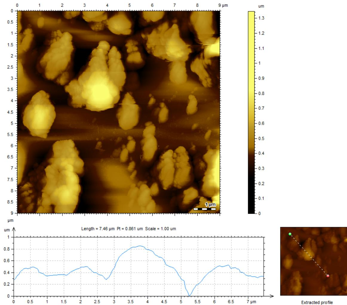
**Figure S13.** AFM image with height profile. Clean ITO slide was soaked in a 0.3 mM Pc8SF solution in toluene for 1 h and allowed to dry. A ca. 400 nm thick film formed with large islands of aggregates.
