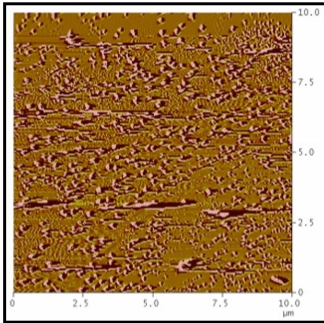
**Figure S10.** AFM image (amplitude, tapping mode) of particles formed by dipping the ITO first in a solution of  $\text{Pc16S}$  and then in a solution of fullerene  $\text{C}_{60}$ .
