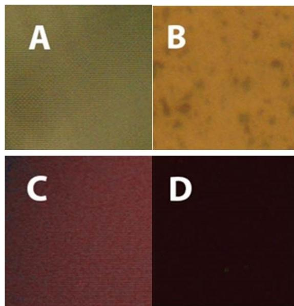
**Figure 15.** Bright field and fluorescence microscope images (each panel  $100 \mu\text{M} \times 100 \mu\text{M}$ ). (A) Bright field image of a film of  $\text{ZnPc8SF}_{144}$ ; (B) Bright field image of a film of 1:5  $\text{ZnPc8SF}_{144}:\text{C}_{60}$ ; (C) fluorescence image of panel A; (D) fluorescence image of panel B. Fluorescence is quenched upon addition of the fullerene.
