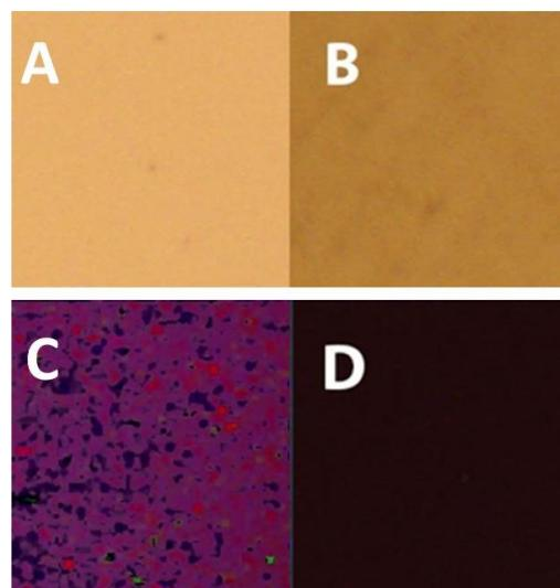
**Figure 14.** Optical and fluorescence microscope images (each panel 100  $\mu$ M x 100  $\mu$ M). (A) Bright field image of a film of ZnPc16SF<sub>288</sub>; (B) Bright field image of a film of 1:1 ZnPc16SF<sub>288</sub>:C<sub>60</sub>; (C) fluorescence image of panel A; (D) fluorescence image of panel B. this shows that the fluorescence of the Pc dye is quenched due to electron transfer to the fullerene.
