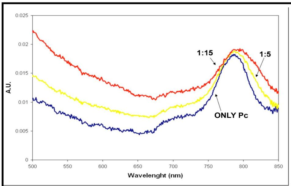
**Figure S7.** UV-visible spectra of a Pc16S film and Pc16S blends with C<sub>60</sub> at different mole ratios on ITO.
