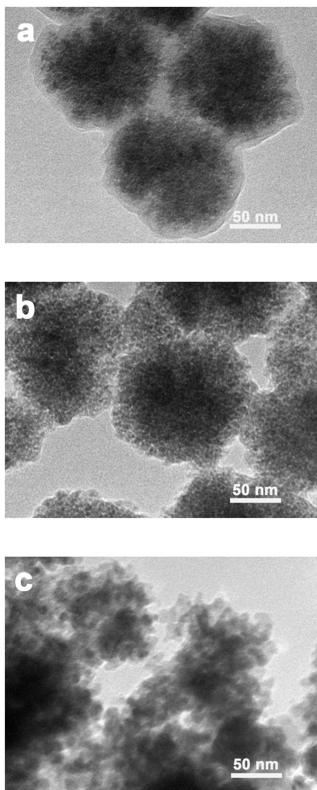
**Fig. S1** TEM images of  $\text{Fe}_3\text{O}_4@\text{AG}$  (a),  $\text{Cit}-\text{Fe}_3\text{O}_4$  (b) and  $\text{Cit}-\text{Fe}_3\text{O}_4@\text{C}$  (c) nanospheres.
