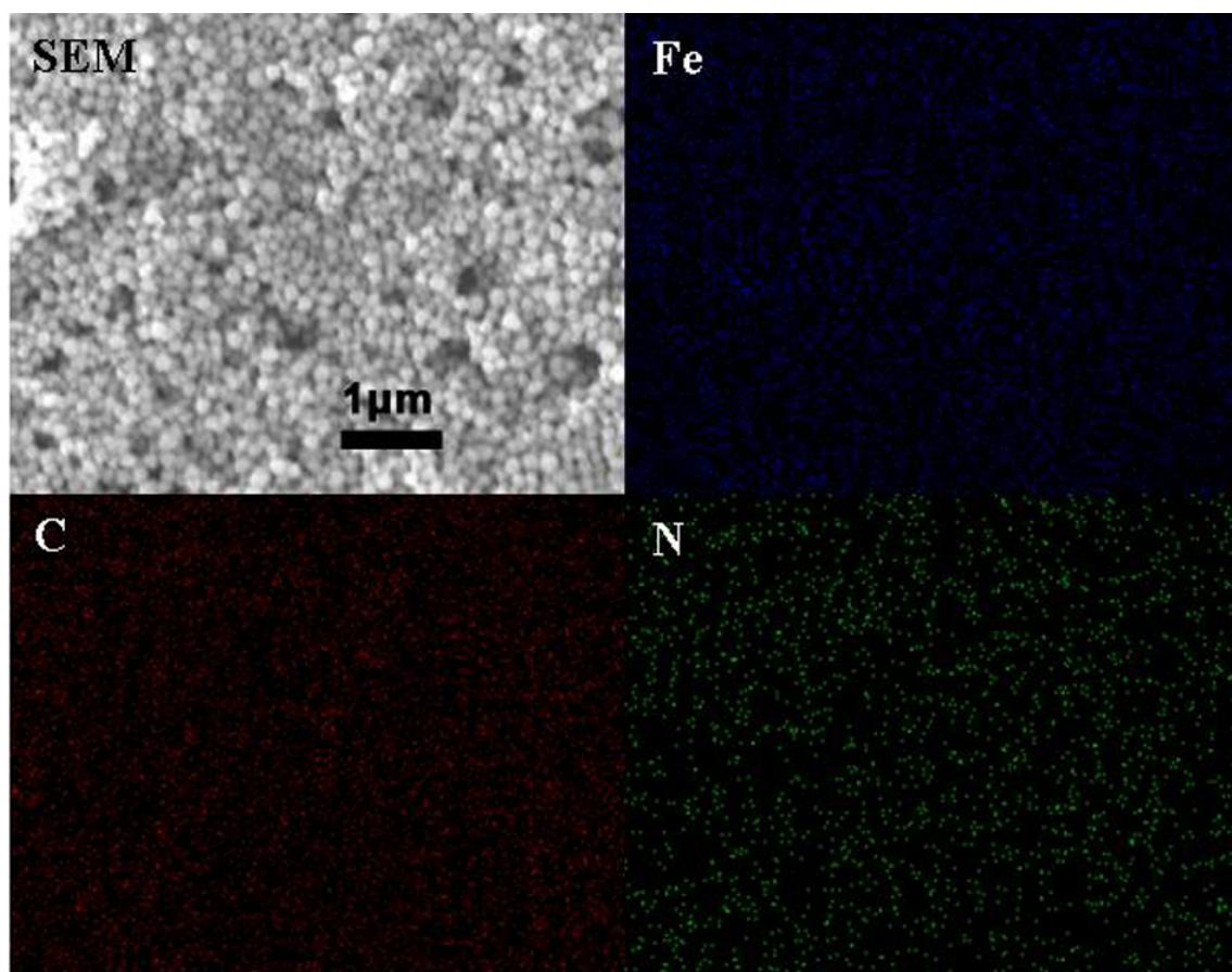
**Fig. S3** SEM image and EDX mapping of Fe, C and N elements of the as obtained N-m $\text{Fe}_3\text{O}_4$ @C nanospheres.
