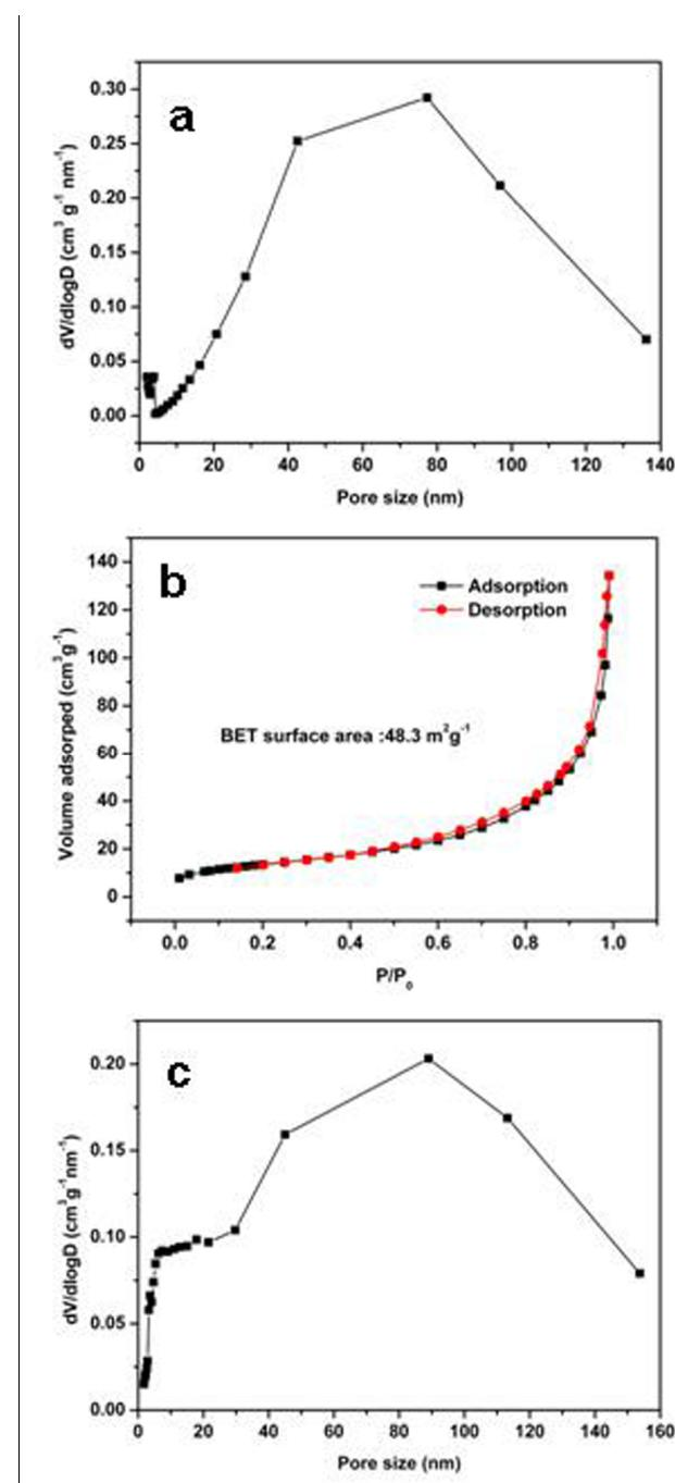
**Fig. S4** Pore size distribution curve of the as prepared N-mFe<sub>3</sub>O<sub>4</sub>@C nanospheres (a); N<sub>2</sub> adsorption-desorption isotherm of Cit-Fe<sub>3</sub>O<sub>4</sub>@C nanospheres and the corresponding pore size distribution curve (b and c).
