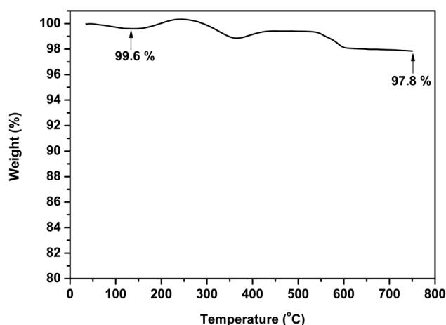
**Fig. S2** TGA curve of Cit- $\text{Fe}_3\text{O}_4@\text{C}$  nanospheres.
