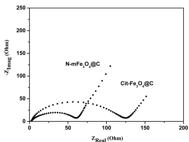
**Fig. S5** EIS of the freshly prepared anodes with  $\text{N-mFe}_3\text{O}_4@\text{C}$  and  $\text{Cit-Fe}_3\text{O}_4@\text{C}$  nanospheres as active materials.
