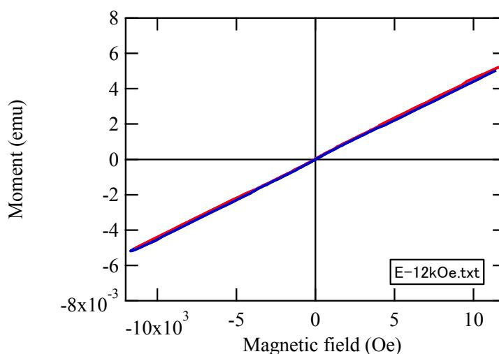
**Figure S2.** Typical magnetization data for Ni/Al LDHs. Magnetic field (H) dependence of magnetization (M) for Ni/Al(3) was measured at room temperature.
