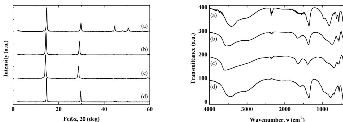
**Figure S1.** XRD profiles (Left) and IR spectra (right) of LDHs.
