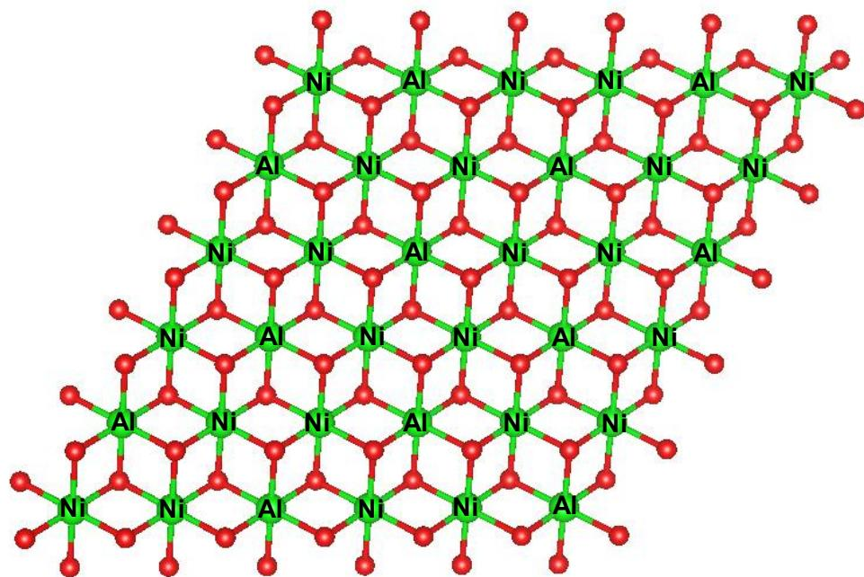
**Figure S3.** Intralayer cation distribution of Ni/Al(2) LDH when Al-O-Al bond is restricted. Oxygen atoms are denoted by red balls. In cases of Ni/Al(3) LDH and Ni/Al(4) LDH, some of the Al atoms are replaced with Ni atoms although the local environment of Al atoms, which are surrounded by six Ni atoms via oxygen atoms, does not vary.
