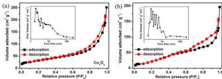
**Fig.S4**  $\text{N}_2$  adsorption-desorption isotherm and the corresponding pore size distribution (inset) of the pre-grow  $\text{Co}_3\text{O}_4$  NWs (a) and the  $\text{Co}_3\text{S}_4$  NSs (b) using BJH method.
