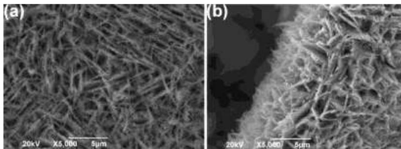
**Fig. S2** SEM images of the sample obtained with the reaction time for 6h under the same condition.
