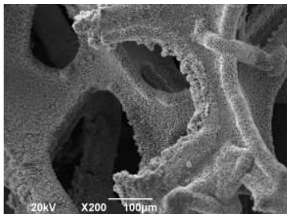
**Fig. S1** Large-scale view of SEM image of the Co<sub>3</sub>S<sub>4</sub> nanosheet arrays on Ni foam.
