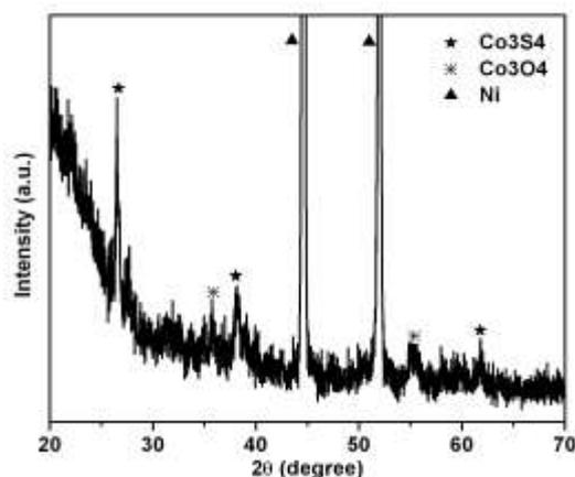
**Fig.S3** XRD pattern of the product obtained for 6 h reaction, indicating that the pre-grown  $\text{Co}_3\text{O}_4$  has been partly converted into  $\text{Co}_3\text{S}_4$ .
