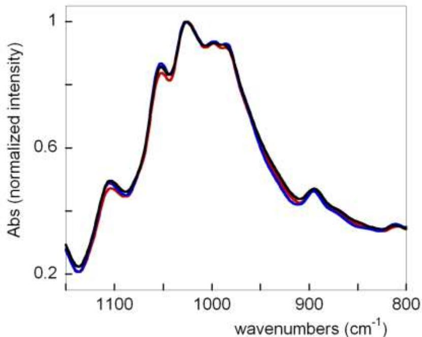
Fig. S2 FTIR ATR spectra of paper. Paper non treated (red line), paper after PEO hydrogel (black line), or PLU hydrogel (blue line) treatment for 45 minutes. The overlap between the spectra suggest that , in both cases, the hydrogels are removed.
