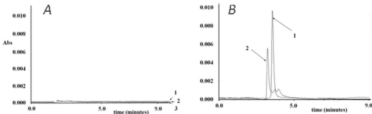
Figure S3 A) HPLC analysis of filter paper (line 1), filter paper treated with PEO gel (line 2), and filter paper treated with PLU gel (line 3) for 45 minutes. B) HPLC analysis of PLU gel (line 1) and PEO gel (line 2)
