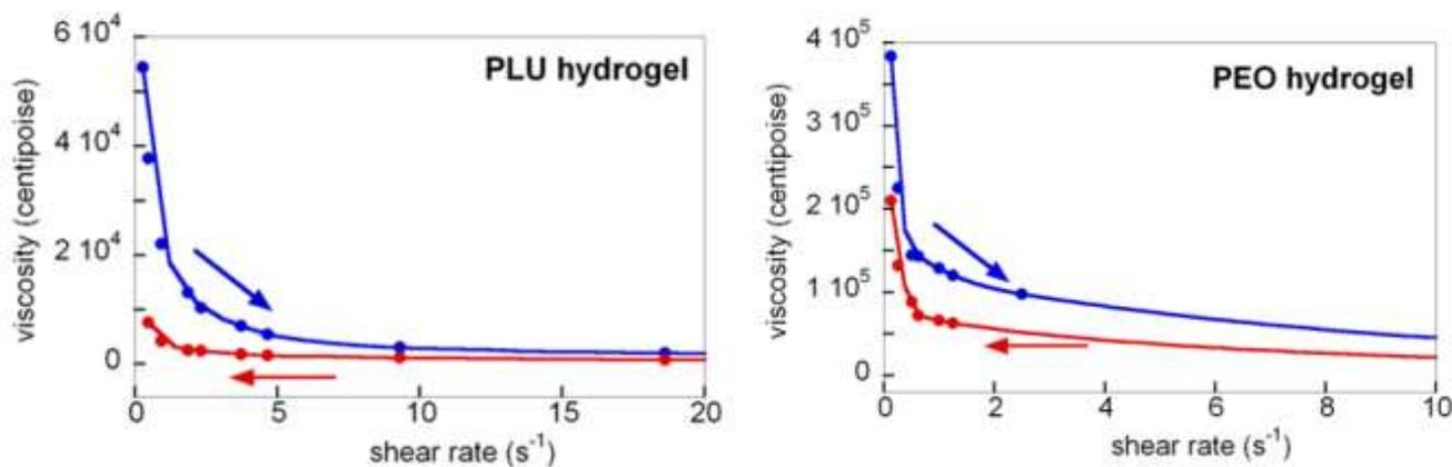
Fig.S1: Viscosity curves of PLU (on the left) and PEO (on the right) hydrogels as a function of a ramp up (blue) and a ramp down (red) of shear rates. The observed differences between the ramp measurements are typical of a thixotropic behavior<sup>15</sup>
