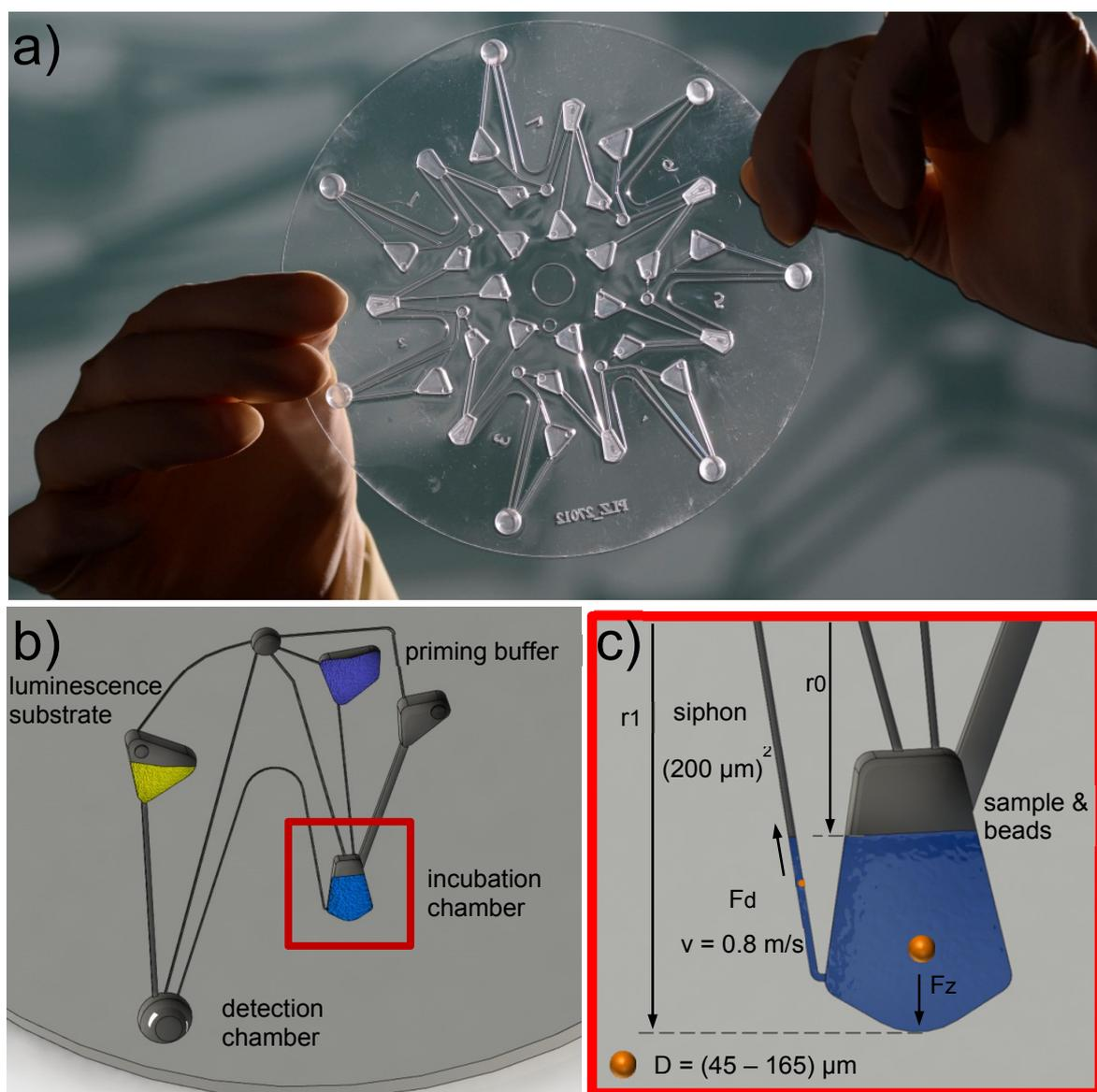
**Fig. S1:** BoNT LabDisk. a) LabDisk comprising seven individual tests; b) design of an individual test. Micro-beads, buffer and sample are incubated in the incubation chamber; and, c) scheme of beads in the incubation chamber and siphon outlet.
