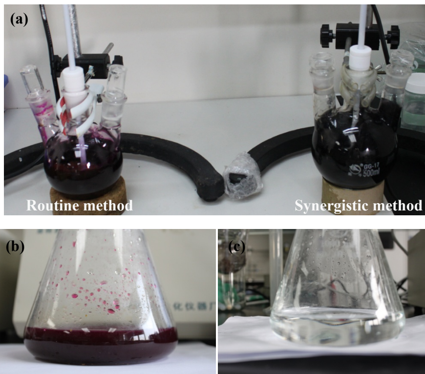
Fig. S1. Photographs of (a) the reaction bottle after adding HCl with 2 min for routine method (left) and 60 min (right), (b,c) below filtrate of the routine method and synergistic method, respectively.
