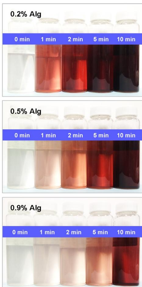
**Fig. S1** AuNPs–alginate aqueous suspensions prepared from alginate solution of different concentrations and SPS discharge times.
