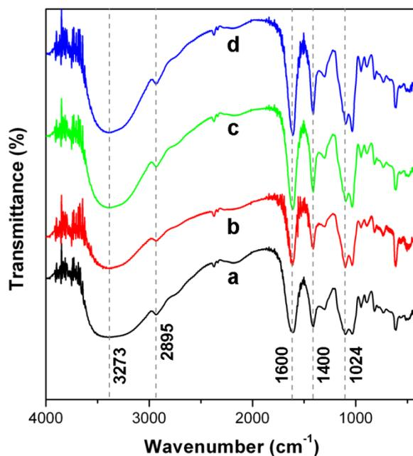
**Fig. S2** FTIR spectra of (a) sodium alginate aqueous solution and AuNPs–alginate aqueous suspensions produced in (b) 0.2, (c) 0.5, and (d) 0.9 %w/v alginate solutions (discharge time = 10 min).
