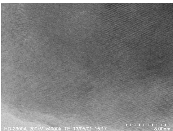
Figure S8. STEM image of a sample prepared with CuCl and HMDST in CH 3 CN at RT for 7 d. This sample consists of fully formed djurleite, and lattice fringes extend in the same direction over significant length scales.
