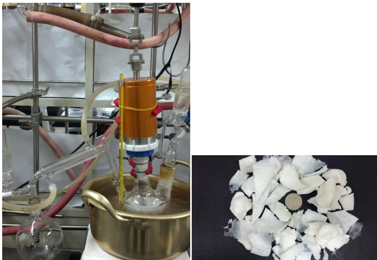
Figure S7. Polymerization apparatus for the scale of 100 g-polymer/batch and the isolated polymers
