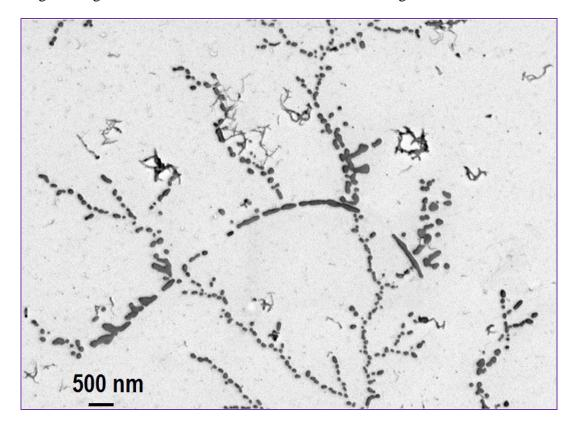
SI-4: FESEM image and EDAX of nanoassembled platform of Ag-PTZH on electrode surface:
