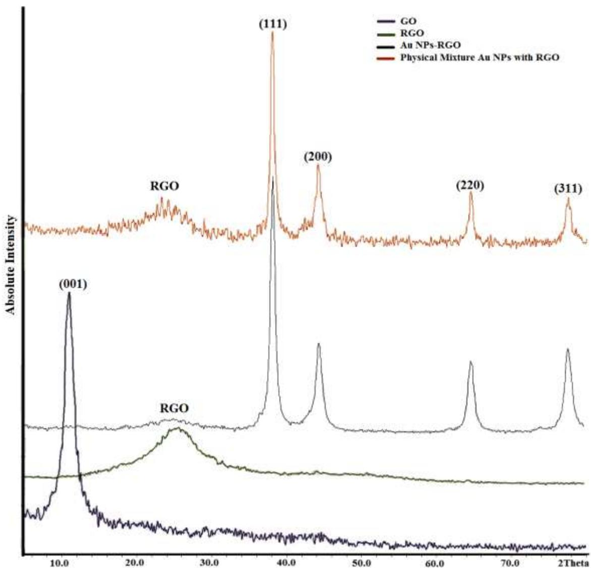
**Fig. S2** XRD patterns GO, RGO, Au NPs-RGO and physical mixture of Au NPs with RGO nanocomposites.
