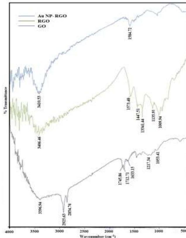
**Fig. S1** FT-IR spectra of GO, RGO and Au NPs-RGO nanocomposite
