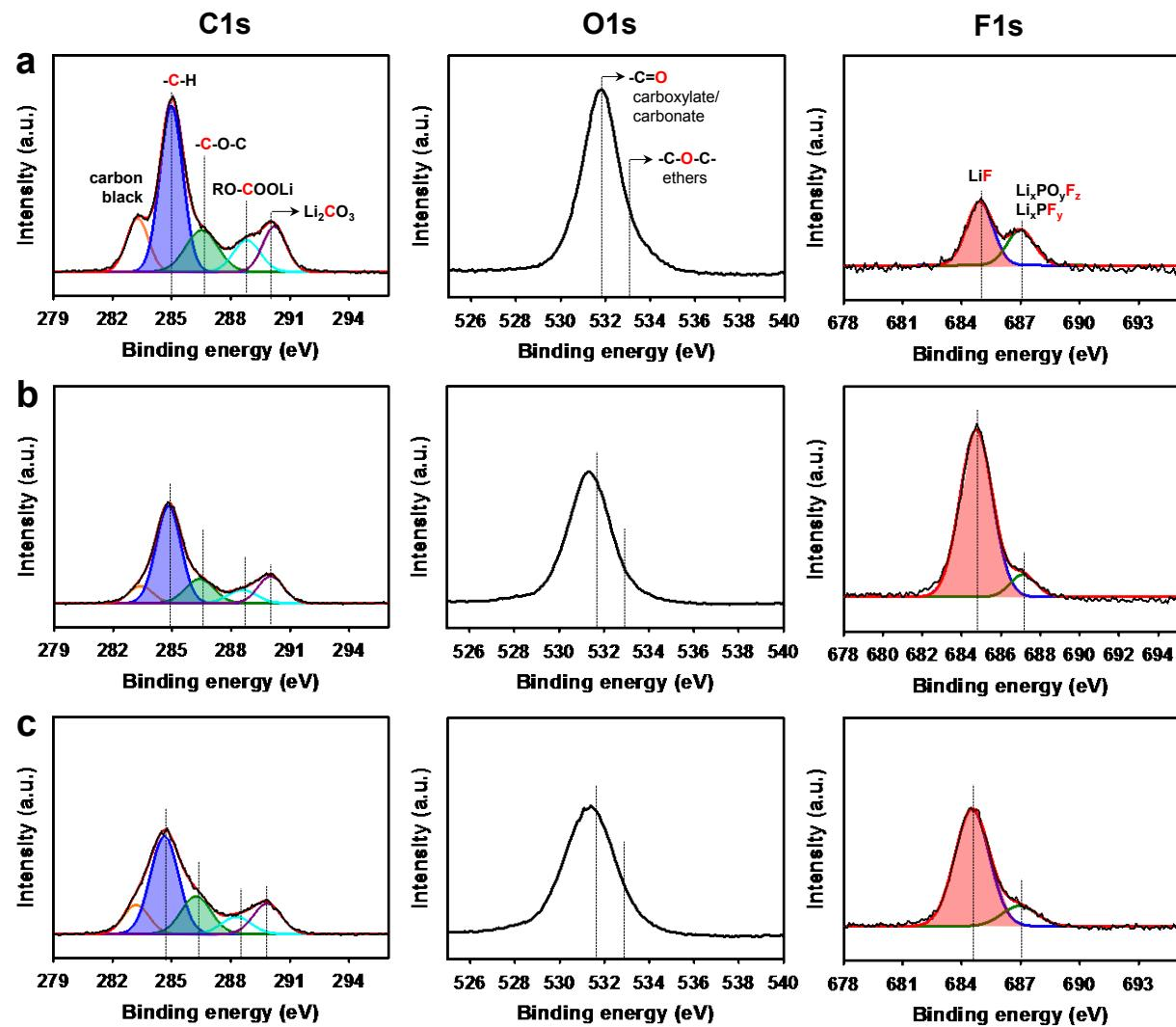
**Fig. S6** C1s, O1s, and F1s XPS spectra of (a) A100, (b) A40, (c) A0 electrodes after first cycle.
