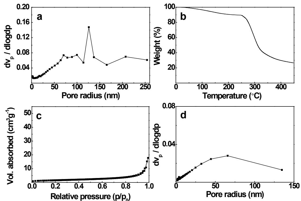
**Fig. S1** (a) Pore size distribution of 3D macroporous Si particles. (b) TGA curve of agarose film.
