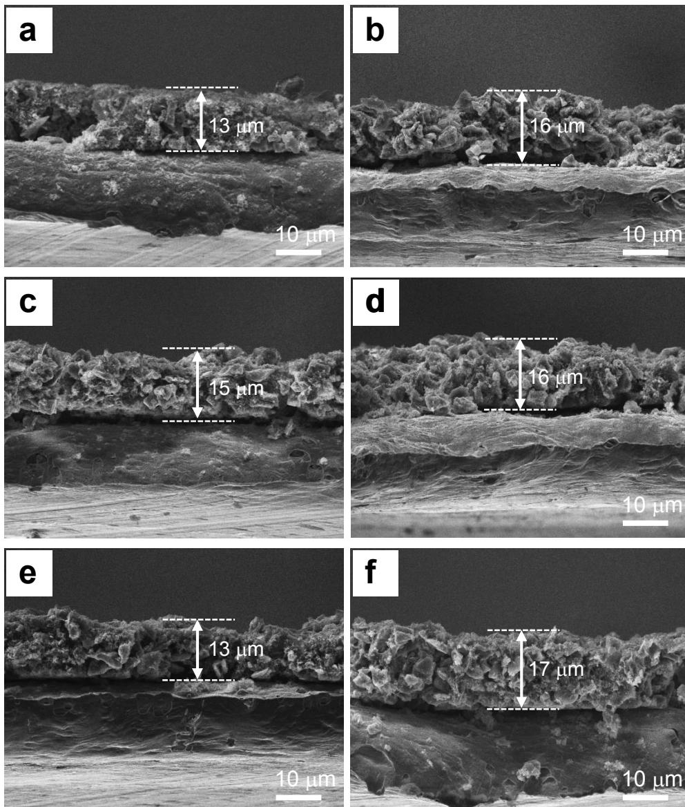
**Fig. S4** Thickness change of electrodes with different binders before and after swelling test in the electrolyte. The pristine electrodes with (a) PAA binder (A0), (c) agarose PAA binder (A40), and (e) agarose binder (A100). The electrode with (b) PAA binder (A0), (d) agarose PAA binder (A40), (f) agarose binder (A100) after swelling test in the electrolyte at 60 °C for 18 hr.
