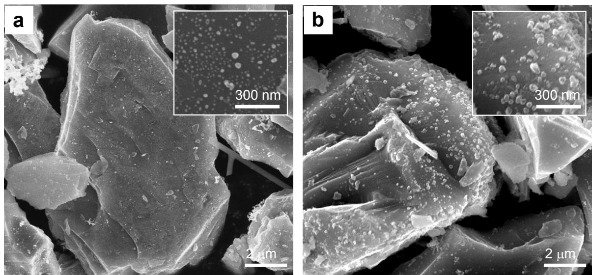
**Fig. S2** SEM image showing (a) Ag and (b) Cu deposited bulk Si particles at the same deposition condition. Cu nanoparticles on the Si surface are much bigger than Ag particles.
