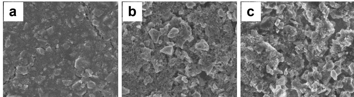
**Fig. S5** SEM image of electrode with (a) PAA binder (A0), (b) Agarose PAA binder (c) Agarose binder.
