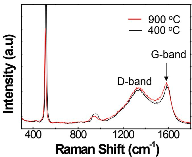
**Fig. S3** Raman spectra of agarose carbonized at 400 °C (black line) and 900 °C (red line).
